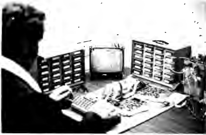
Mike is demonstrating the prototype Sphere system. It is on three boards, a keyboard/character generator, CPU and memory board. The output is being displayed on a small television screen.
