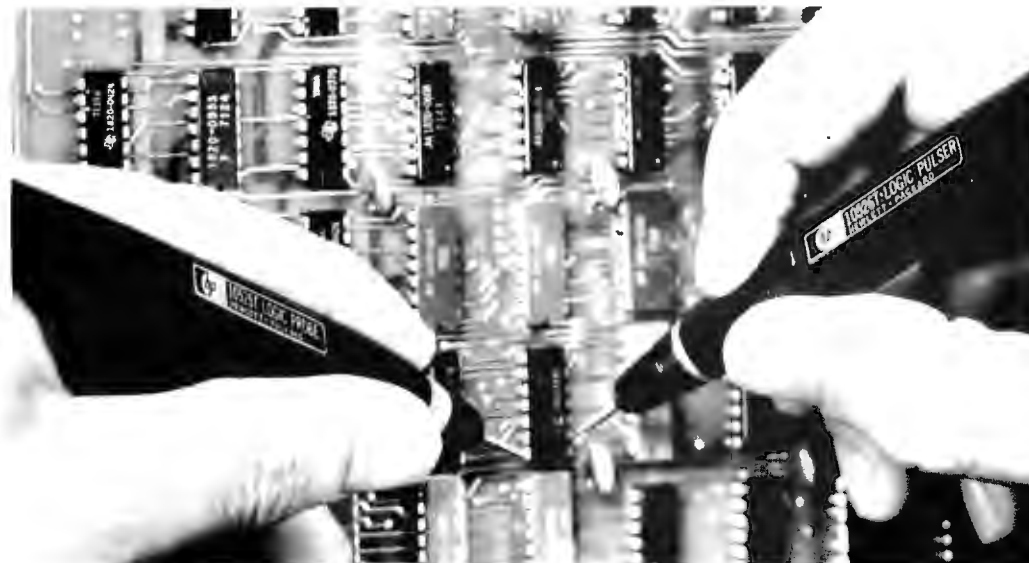
The Hewlett Packard 10525T logic probe and 10526T pulser.
