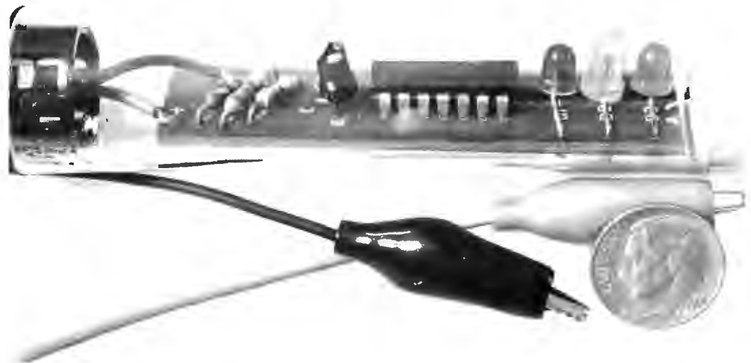
A detail of the Chesapeake Digital Devices logic probe board. The three LEDs are at the right in this picture, with the 74S00 IC in the center.
