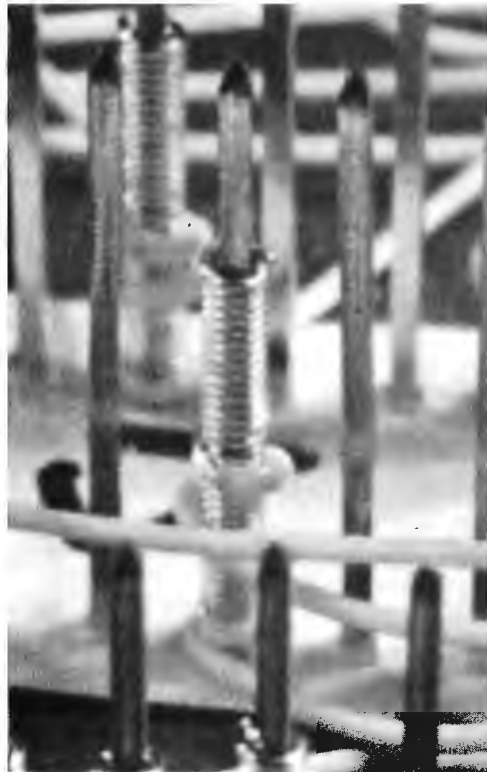
Photo 1: One of the most widely used custom assembly methods in the computer industry is wire wrapping. Special square wire wrap posts are built into sockets or mounted directly onto components. The stripped ends of insulated wires are connected to the posts using a special electric or hand operated tool. The result is an excellent connection with gas tight "vacuum welds" at each corner of the post as the sharp edge cuts slightly into the wire. Wire wrapping is a quick, easy and permanent way to connect point A to point B in your custom circuitry.
