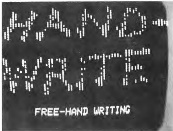
Photo 3: The light pen can be used in an "enhance" mode by using a footswitch control to flood the screen momentarily when the light pen is in position.
