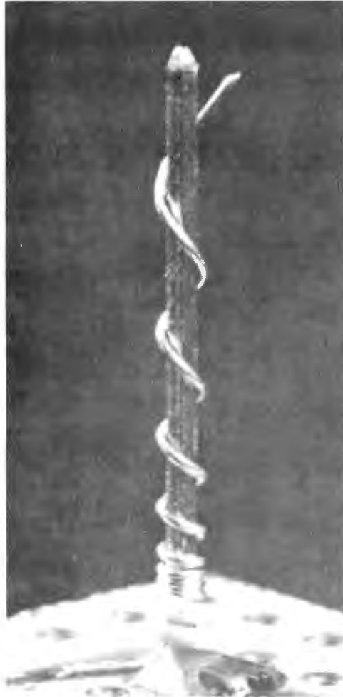
Photo 6: Continuing on the theme of less than optimal wrapping results, this picture shows an example of the "impatient wrap." The primary cause of the impatient wrap is your own impatience to see the result. If the wire wrap gun is removed from the post while the wrapping action is under way, the result will be widely spaced coils of wire often covering the length of the post. This example is an exaggerated version concocted on purpose; the typical case is a normal base to the coil with the top one or two layers spread out. The solution to this problem is to allow the gun to do its work before removing it from the post. In a case such as the one shown here, removal of the connection and rewinding should be done. In milder forms of the impatient wrap, the wrap would not necessarily have to be replaced.
