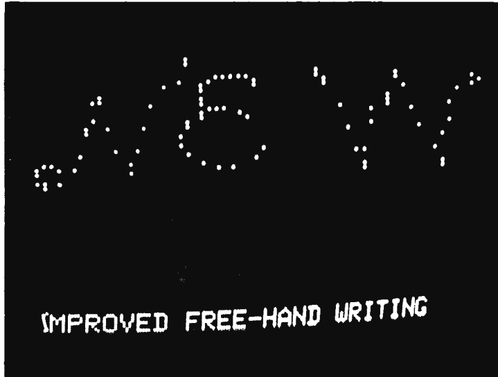
Photo 7: Using the improved circuit of figure 3 reduces much of the over-writing of multiple dots which occurred using the original circuit of figure 1. This is an enhance mode picture.
