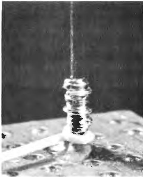
Photo 5: To quote the previous caption, "When the trigger has been pulled on a loaded wire wrap gun, the result (hopefully) will be a perfect wrap every time." Here is an example where hope was in vain. A problem which sometimes occurs is the "wrat's nest" wrap shown in this photograph. The normal operation of the wrapping gun includes retraction of the bit inside the sleeve as the wire layers are added to the coil around the post. A spring loaded mechanism in the gun provides for this controlled retraction. Occasionally the bit sticks and does not retract properly. This results in a jumbled mess as layers of wire wrap over previously wrapped layers. If the wrat's nest wrap occurs only occasionally, the likely cause is your tool position while wrapping. If the bit is not centered about the wrapping post, friction in the pilot hole can prevent the bit from retracting properly. If the wrat's nest wrap occurs consistently a likely cause is dirt and grime buildup on the bit. If particles of metal scraped off the wire are allowed to accumulate, the resulting friction can inhibit retraction of the bit. Thus if the gun consistently makes wrat's nest wraps, removing the bit and cleaning it may resolve the problem. After cleaning, the bit may be oiled. Oiling should be done very sparingly at the gun end of the bit so that excess oil does not get in the groove and onto the wire. When a wrat's nest occurs, whatever the cause, good practice indicates that you should remove the mess and start over.
