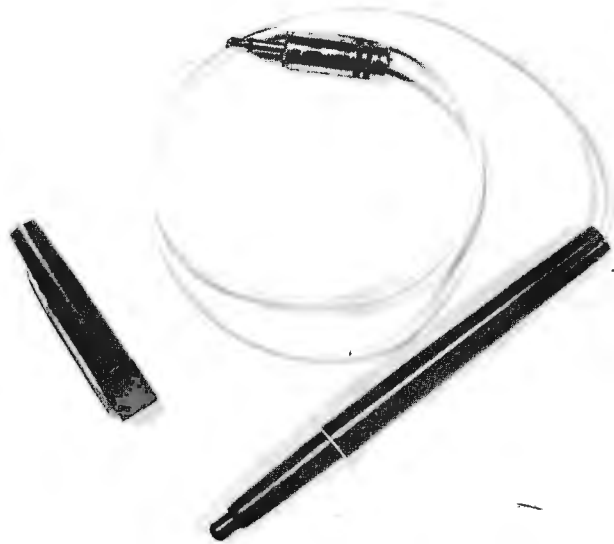
Photo 4: This shows a pen based on the TI type L-63 photocell, built using a marking pen case.
