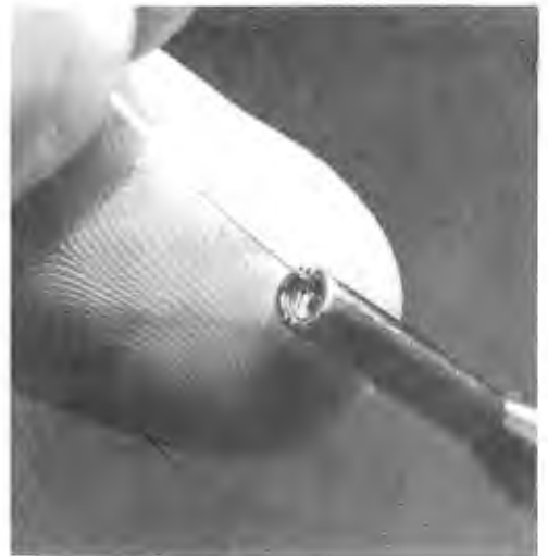
Photo 2: The business end of an industrial quality wire wrap tool is the bit and sleeve assembly. The bit is driven by a high speed motor (or hand operated mechanism) and rotates around the post to be wrapped. The center of the bit has an alignment hole which fits over the wire wrap post to guide the operation. The bit also has a groove along its length into which the stripped end of a wire is inserted as shown. The wire is held in the groove by the sleeve and is pulled out during the process of wrapping. The sleeve itself does not rotate and is held rigidly in position.
