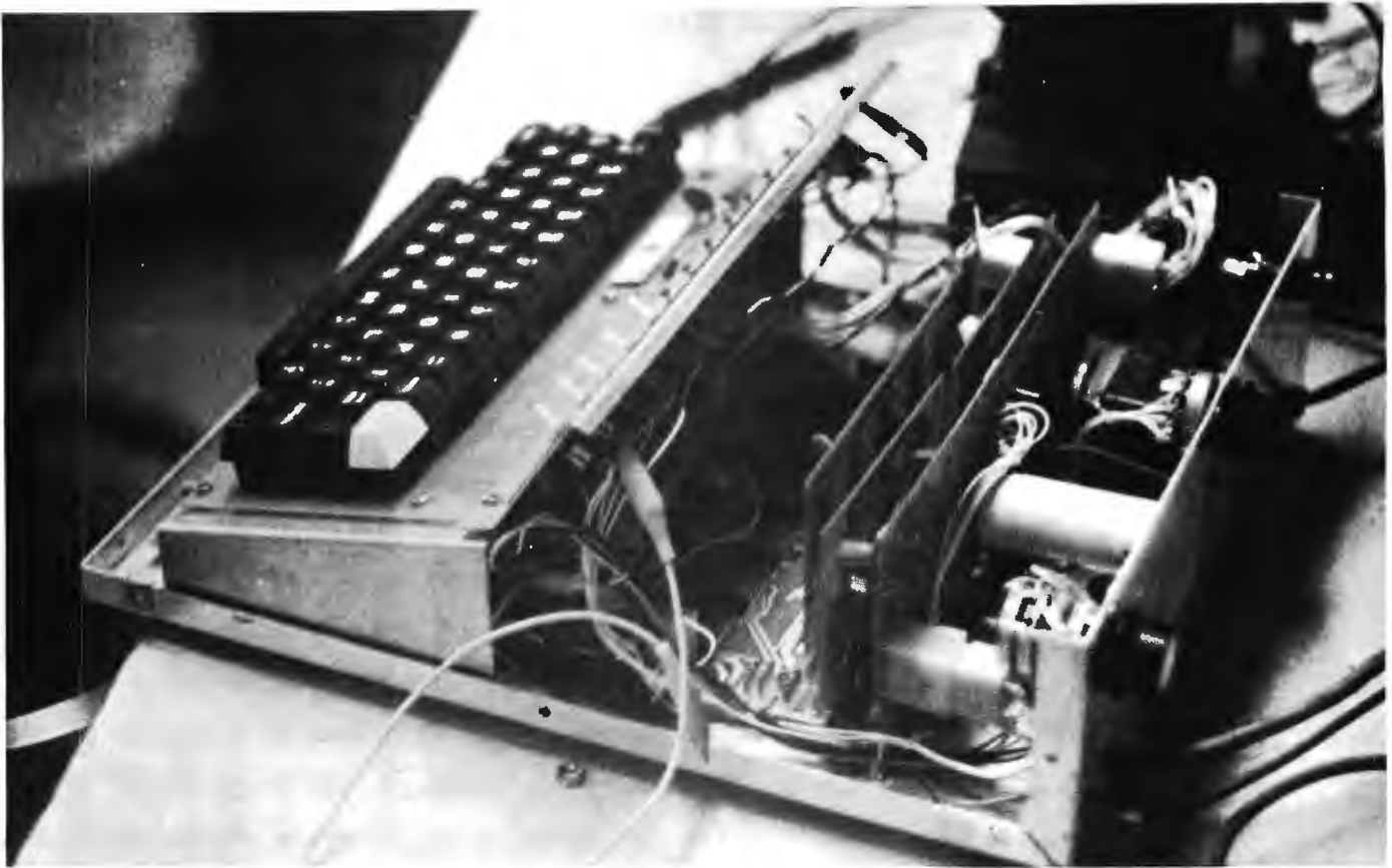
Southwest Tech CT-1024 video terminal . . . built on a homemade base. Row of switches along the top is for extra functions.
