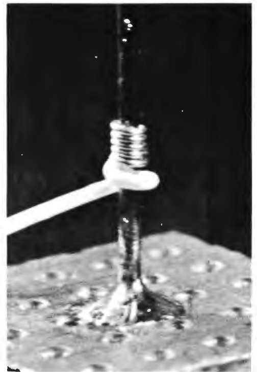
Photo 7: The length of the coil produced by the wrapping action is a function of the length of bare wire prepared for insertion in the tool. For the typical .025 inch square wrapping posts with 30 gauge wire, approximately 8 layers will be added to the coil for each inch of bare wire inserted into the bit. This photo shows an example of the "pigmy wrap." When a short coil of wire is produced, one possible explanation is that not enough wire was stripped when preparing for the connection. (Another possible explanation is that the wire broke, leaving most of the stripped section inside the groove where it must be removed by disassembling the tool.)
