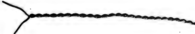
Photo 3: Twisted pair cable is the only good data transmission line which can be easily fabricated at home. Here is an example made using an electric drill to do the twisting.
