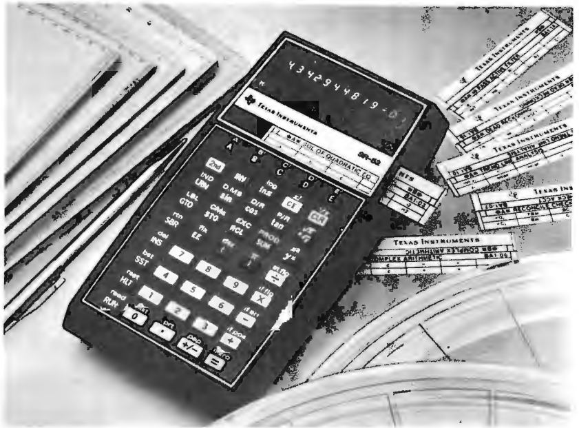
Photo 1: The SR-52 Calculator. Like its cousins in the microcomputer and large computer world, the SR-52 has magnetic recording features allowing the user to purchase and build a library of software.
