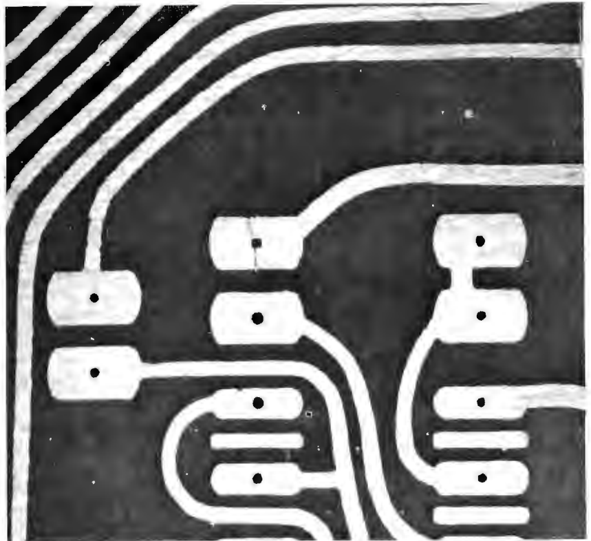
Photo 8: Close up, a successfully etched printed circuit will have even lines with no hairline cracks or other imperfections. This example shows such a result, prior to drilling out the holes for component leads.
