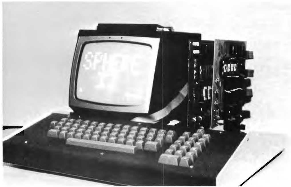
Photo 3: It works! Here is my completed Sphere system in operation driving a small video monitor (not purchased from Sphere). The board interconnections are made with flat ribbon cables, and the keyboard is shown mounted in its case.
