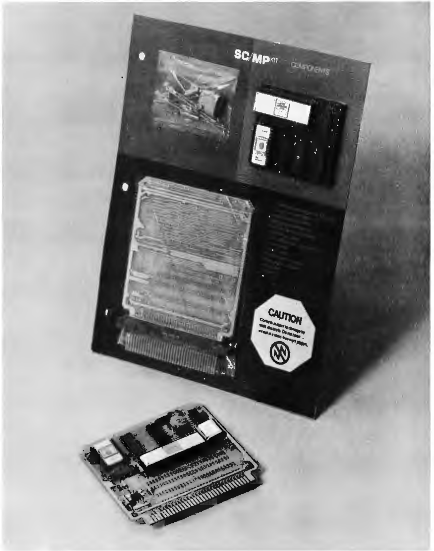
Photo 1: National Semiconductor markets an evaluation kit for SC/MP which is probably one of the least expensive ways to try out a working processor. The kit includes the circuit board, all electronic components including processor and firmware ROM, crystal for 1 MHz clock speed and power supply regulator. The assembly of this board, using ample documentation as a guide, results in a computer with 256 bytes of programmable memory, a 512 byte firmware operating system called "KITBUG" and a 20 mA Teletype current loop interface for operator control. A single 12 V power supply is required.
