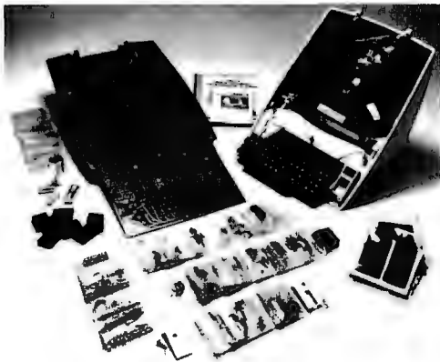
Photo 1: ADM-3 kit shown in a "beauty contest" arrangement. The resulting terminal looks like the photo found on page 96 of June 1976 BYTE , but beauty in the eye of a kit builder is in the arrangement and packaging of the parts plus documentation.
