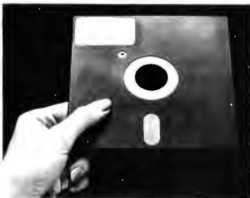
Photo 2: The new Shugart minidiskette is exactly the same as its larger counterpart, the standard flexible disk, except the size is only 5.25 inches (13.3 cm) square. Minidiskette media comes soft or hard sectored and stores 109.4 K bytes of data (unformatted), or 3125 bytes per track. The media is available from Shugart and several independent media suppliers.
