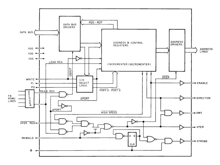
Figure 11: Block diagram of the 3854 direct memory access.
