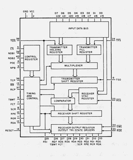
denoted by the various signal lines. Figure 5 shows a block diagram of the S2350, along with captions detailing these lines and their relation to the interface as a whole.
