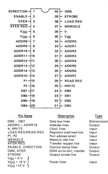
Figure 10: Pin designations for the 3854 direct memory access chip.
