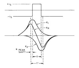
Figure 4: Merging of transitions. When two transitions come close together on the tape, the response curves (see figure 2c) upon reading the data can overlap significantly. This crowding of flux changes tends to cause interference such that the amplitude of the signal is reduced, and the time coordinate of the peak of the curves will shift slightly.
