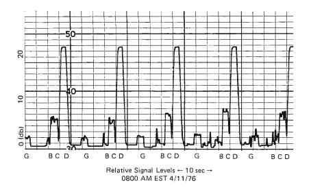
Figure 4: Signal envelope from the Mini-O receiver at 10.2 kHz. This is a photo reproduction of a strip chart recording made from data taken at 8:00 AM EST on April 11 1976.
