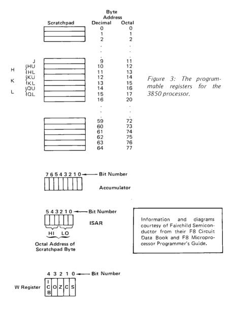
8 bit general purpose registers that are addressed by a 6 bit indirect scratchpad address register as shown in figure 3. The W register, a 5 bit status register, indicates sign, carry, zero, and overflow conditions as a result of various processor operations and contains the interrupt control bit. The processor chip also contains two 8 bit, bidirectional, IO ports with output latches for transferring data to and from the processor.
