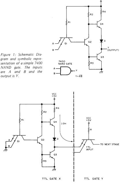
Figure 2a: Schematic Diagram of a basic TTL gate showing the direction of IOH when the output is high, VOH.
