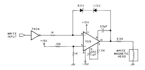
Figure 3: A typical head drive circuit for saturation recording. The 709 operational amplifier here is used to drive the magnetic tape head to saturation in either direction by applying a 10 V signal with respect to ground. A magnetic recording head winding resistance of typically 100 ohms in the digital cassette case results in a current of 10/3400=0.003 A (3 mA).
