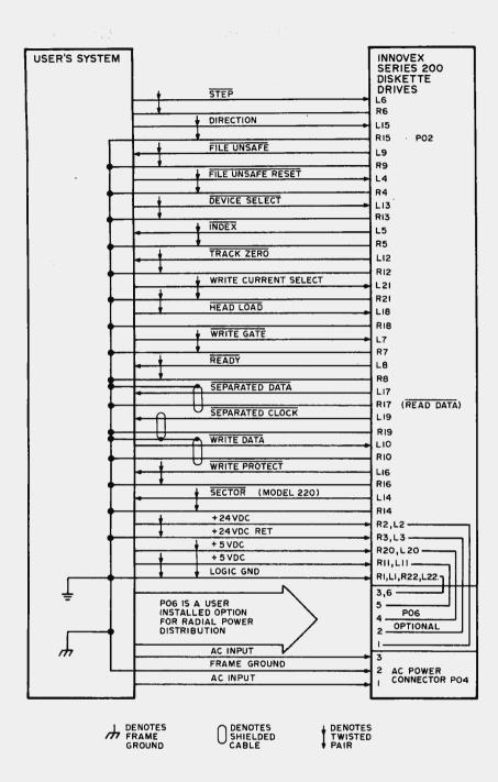
Figure 1: This diagram, redrawn from the Innovex Series 200-M Maintenance Manual, shows all of the TTL level signal lines that must be passed between the disk drive and the controlling interface. The signals sent to the drive from the interface are:
