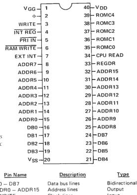
Figure 6: Pin designations for the 3852 dynamic memory interface chip.
