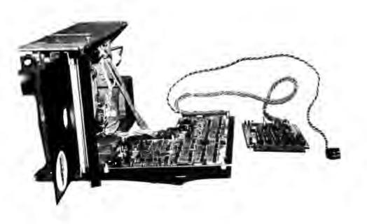
Photo 1: The author's disk drive and interface board shown removed from the system. The Innovex drive is at left, with a diskette partially inserted in the front door and the electronics board for the drive shown in an "open" position. The interface board is at the end of a multiconductor twisted pair cable, and a separate cable is used for drive power.
