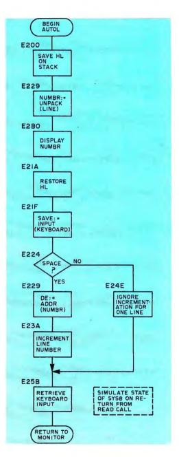
Figure 3: Flowchart of the AUTOL routine that increments the line numbers and determines if an executive command has been entered. If an executive command is input the automatic line numbering will cease. Addresses in this figure refer to listing 3.
