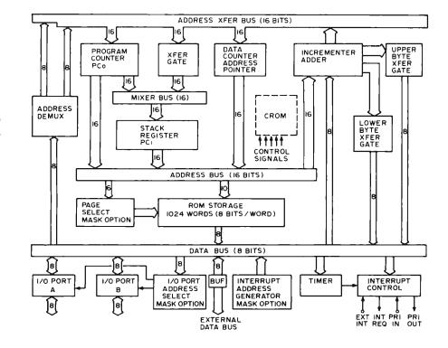
Figure 5: A block diagram of the 3851 program storage unit.
