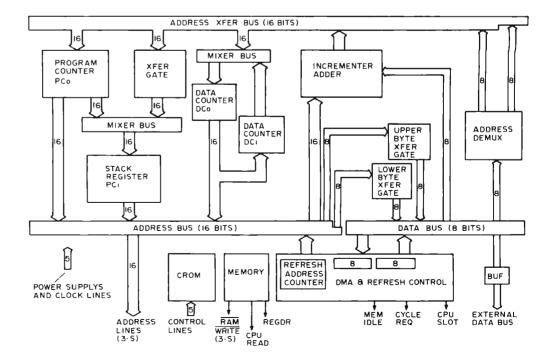
*Figure 7: Block diagram of the 3852 dynamic memory interface.*  pull up. The programmable timer and interrupt logic are accessed in the same manner as the IO ports with specifically assigned port addresses that are the same in each program storage unit except for the page select bits.
