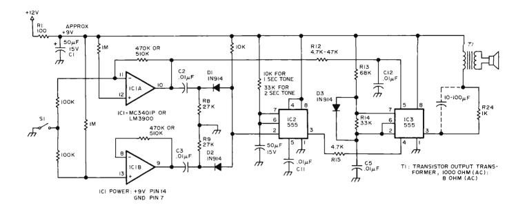
Figure 1: One way of producing audible tones on command. The input is shown as a switch, S1, at the left but could just as well be a signal derived from a single bit computer output. of the desired tone burst. The high frequency bypasses, C11 and C12, keep the circuit from being triggered or modulated by RF noise that is present on VCC and ground.
