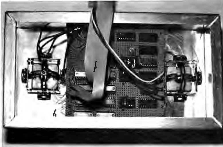
Photo 2: Underside of finished assembly showing wire wrap board and two joysticks.
