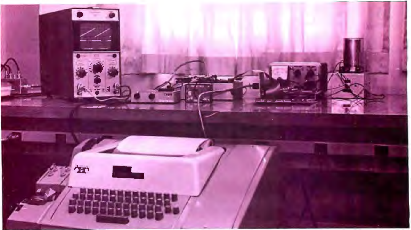
Photo 2: Mini-O in operation on the bench. The setup shown here uses a Teletype Model 33 ASR with the JOLT computer (at right in front of power supply), and the Sinclair clock reference (in front of interface box on bench). The display on the oscilloscope shows output from a lines of position digital to analog conversion output described (in concept) in part 1 of this article.
