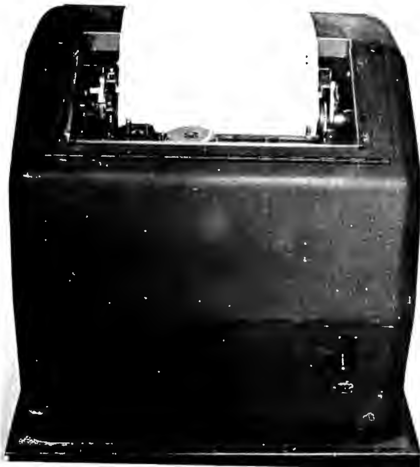
Photo 1: A Teletype Model 15 RO printer. This "receive only" model is shown with cover removed (above) and with the cover in place.
