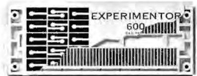
Both models feature 94 five-point terminals (vertical lines) and two 48-point bus strips (one strip shown).
