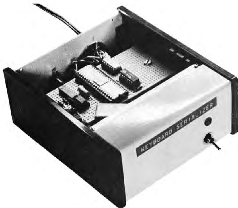
Photo 2: The Remote Transmitter Assembly. The transmitter also needs a power supply, contained within this box, for both itself and the keyboard. With a stylish cabinet such as this, you can be proud to display your newest addition to your friends.
