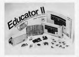
the read only memory contains routines for servicing interrupts, program transfer to and from cassettes, tape searching programs, and a program to test the finished kit. The executive program uses 14 bytes of the programmable memory as a scratchpad memory, leaving 114 bytes for user programs. An optional 128 bytes of programmable memory can be added later.
