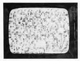
field, obtained by the application of power to the memory. Each chip has a preferred start-up value, so this pattern tends to be the same whenever one turns on the display. In this picture, blanking has been suppressed, so the distortion due to nonlinearities at the top of the screen is quite visible.
