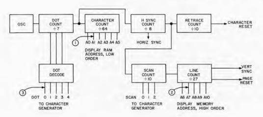
Figure 1: Block diagram of a television display. This version is very similar to the display described by C W Gantt in June 1976 BYTE, page 18. The points indicated by circled numbers are used as described in the text to generate the various test patterns shown in photos 2, 3, 4 and 6.
