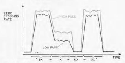
Figure 4a: A plot of the word "SIX" showing the zero crossing rate as a function of time. The word is shown split into its four phonemes. In this case, the signal is first processed through two bandpass filters. The number of zero crossings is then determined by the computer. Results for both filters are shown. As the graph indicates, there is a very short period of silence during the pronunciation of the KX phoneme which can be verified by slowly pronouncing the word "six."
