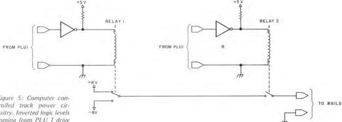
Figure 5: Computer controlled track power circuitry. Inverted logic levels coming from PLU 1 drive two types of relays. The first type (represented by relay 1 in this illustration) chooses the polarity of the voltage going to the track, while the second type (relay 2 here) applies power to the track. Only certain strategic areas of the track require polarity switching.
