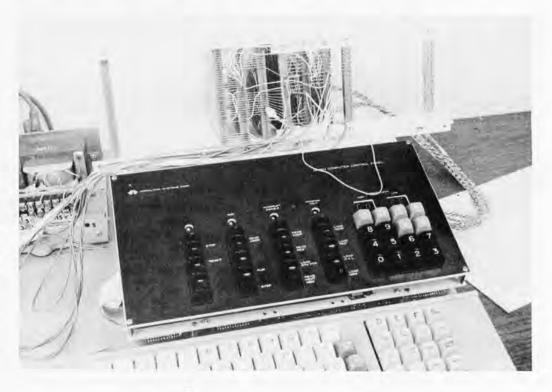
Photo 7: Physical layout of the equipment. The author's display is shown here as it was built on prototyping cards with a bus wired backplane between connectors. The clip lead is shown here attached to memory address bit 7, as used to generate photo 3. The computer and keyboard are in the foreground.
