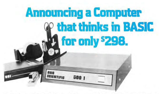
Ohio Scientific's new Model 500 computer has full mini-computer BASIC in ROM and a minimum of 4K RAM for user programs. BASIC is always there when the computer is turned on.
