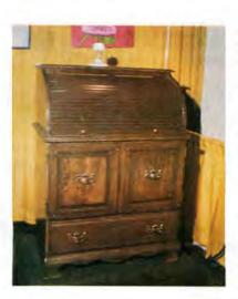
Photo 2: The mild, unassuming roll top desk at the left of this sequence hides an intelligence. For, when all the doors and slides of this "desk" by RDC Enterprises (8352 Stanford Av, Garden Grove CA) are opened, they reveal an experimenteroriented computer with built-in Altair bus extender card at desk level, a keyboard at desk level and video monitor. The actual computer mainframe is below desk level behind doors, and the bottom drawer can hold the experimenter's tools.
