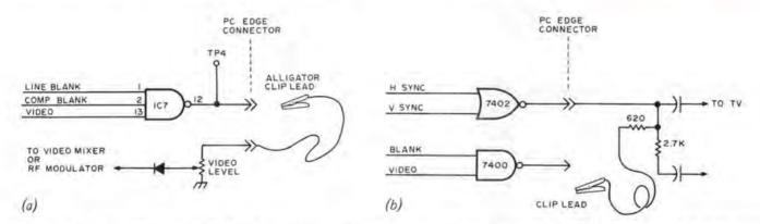
Figure 2: (a) A modification of the Gantt televison display circuit, of page 18, June 1976 BYTE, to use this test instrument technique. The line from IC7 pin 12 to the video level potentiometer is broken so that input to the video mixer, and thus to the TV, is taken from some arbitrary point under test rather than the usual source. (b) The author's video output circuitry, with a similar clip lead jumper normally in place for display purposes, but free to be moved around for testing purposes.
