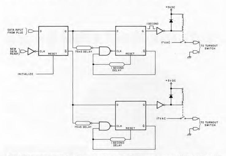
Figure 8: Coil activation circuitry. The coils used to energize the track solenoids cannot be energized 100% of the time (a 100% duty cycle) without burning up. This circuit uses flip flops and delay elements to provide a one second pulse to a relay where it is converted to 17 VAC, sufficient to activate the solenoid. This illustration, like the rest in this article, is intended to illustrate a concept rather than to serve as a basis for actual construction.
