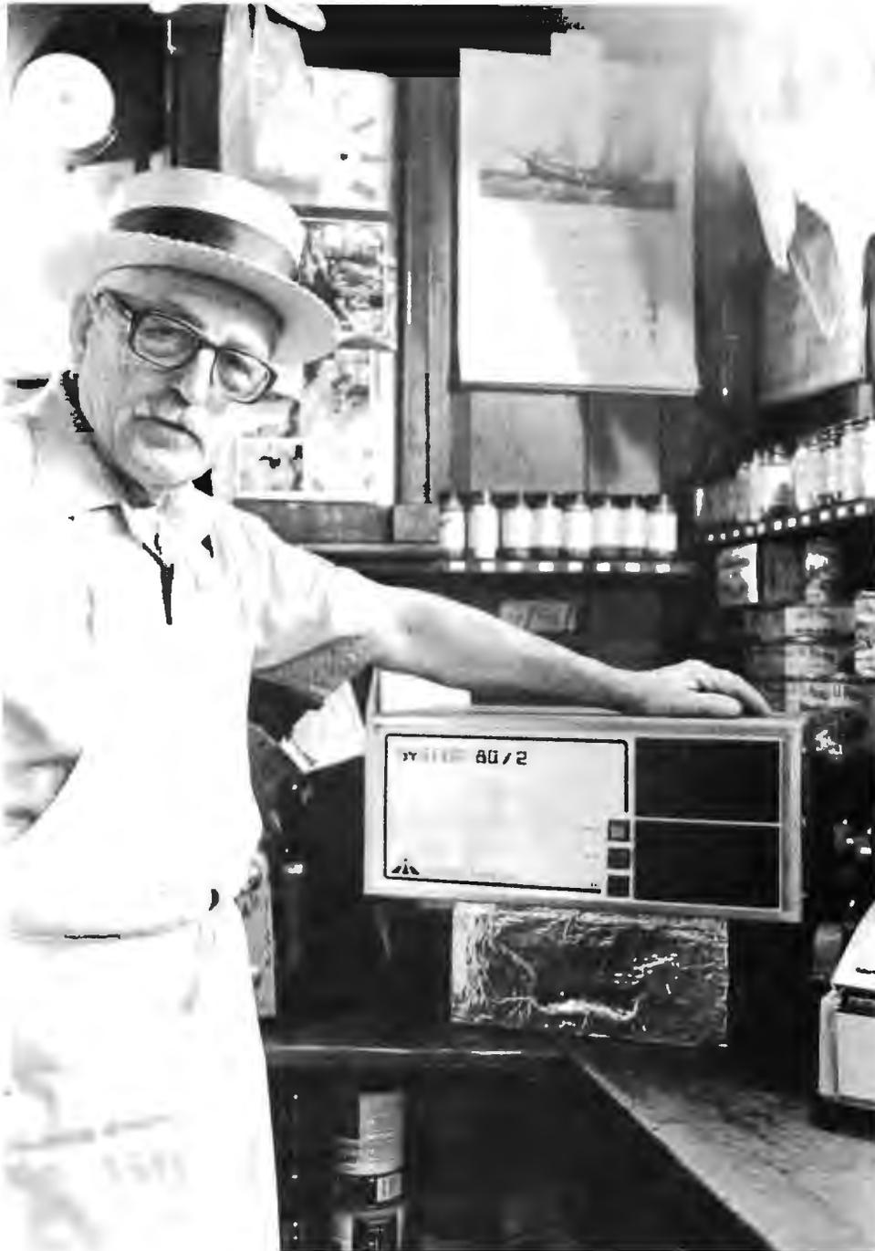
Whether managing accounts at the local general store or aiding in the development of the latest Space War, the **MiniTerm Dual MiniFloppy\* System 80/2** can do the job best. Z-80 powered, and S-100 bus structured, the **System 80/2** mainframe with regulated supplies for two mini floppies\* is also available without cards and drives.
