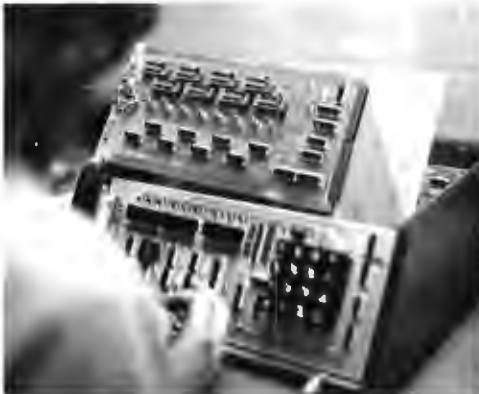
Photo 3: Here is an H8 computer used in a production and test situation at the Heathkit plant, with its memory board mounted on an extender. The boards in the H8 are mounted at an angle with respect to vertical, which keeps the height of the cabinet down while allowing bigger boards to be designed.
