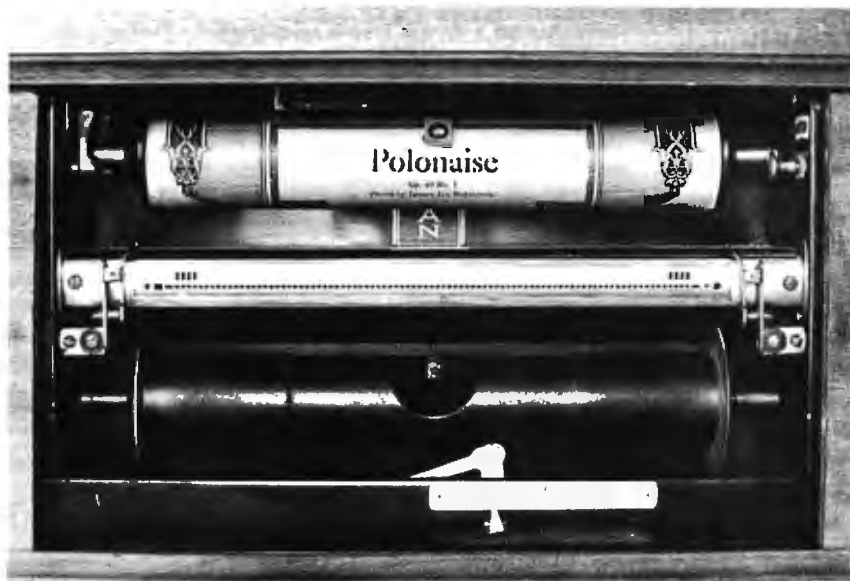
Photo 2a: The spool box, showing the brass tracker bar. There are 88 holes across the bar, corresponding to the notes of the piano. There are additional holes at each end to input two 4 bit "nybbles" of information to the dynamics (volume) control system from the paper roll.
