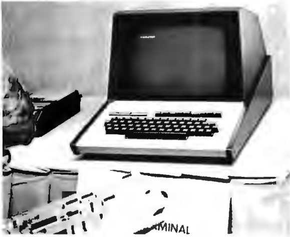
Photo 1: Perhaps a key element of the Heath line is this H9 video terminal, used with either the H8 or H11 systems. It is a full ASCII terminal (but with upper case only in the display section) and a wide range of data rates.
