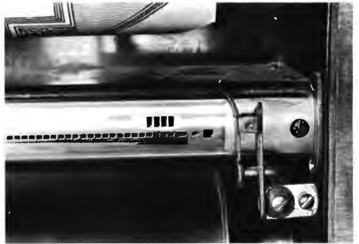
Photo 4: A closeup illustrating the four right hand dynamics control holes, located slightly above the center line of the rest of the holes.
