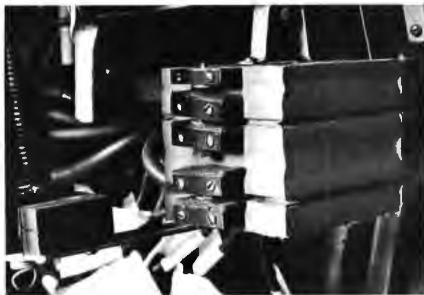
Photo 3b: The accordion pneumatic shown converting the integer value 10 into one of 16 possible mechanical positions. This corresponds to the binary number 1010 on the roll. See photo 5.
