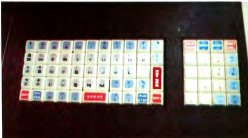
Photo 2: A closeup of the PET's unusual touch-sensitive keyboard with 73 keys and 64 shifted graphics symbols in addition to ordinary upper case ASCII characters.
