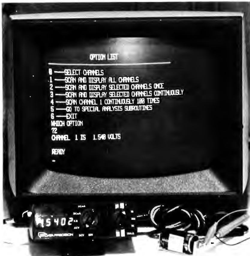
Photo 4: An illustration of the accuracy of the computerized voltmeter. A Data Precision 4½ digit digital multimeter and the author's system simultaneously measure a C cell battery. The computer value is 1.540 V compared with the Data Precision reading of 1.5402 V.
