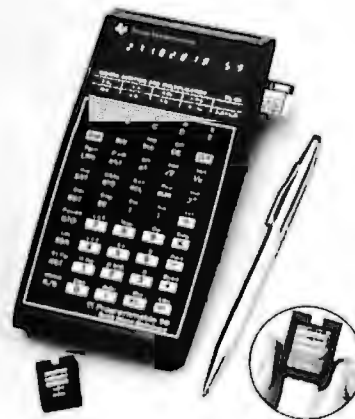
Photo 4: The TI 59 features Solid State Software plug-in program library modules of up to 5000 program steps, as well as a magnetic card reader and internal memory for 960 program steps.
