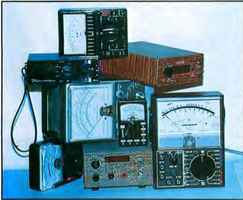
Photo 2: Eight meters (some are multimeters, others are voltmeters) which could be replaced (at least for DC voltage measurements) by the computerized 8 channel voltmeter described here.
