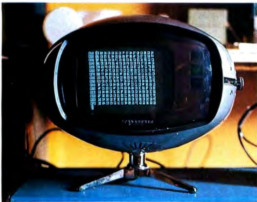
Photo 2: The SOL's display generator produced this video character graphics pattern on the author's television monitor.
