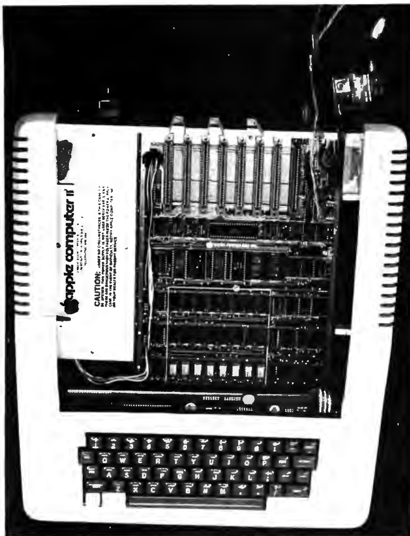
Photo 3: Removing the cover and looking straight down into the unit, the major internal subassemblies can be seen. At the left is the proprietary switching power supply unit; at the right along the bottom of the cabinet is the main processor board, with room for 48 K bytes of programmable user memory (using 16 K memory parts) and an 8 slot IO bus used to interconnect peripherals. At the right toward the rear of the cabinet (top of photo) is the RF modulator used to drive the television on channel 3. The keyboard can be seen toward the lower edge of the photo.
