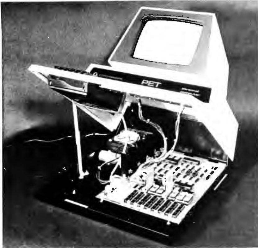
Photo 5: The PET props open for easy service access. Besides the main printed circuit board, the unit contains a TV chassis type circuit board and a third board in the cassette recorder.
