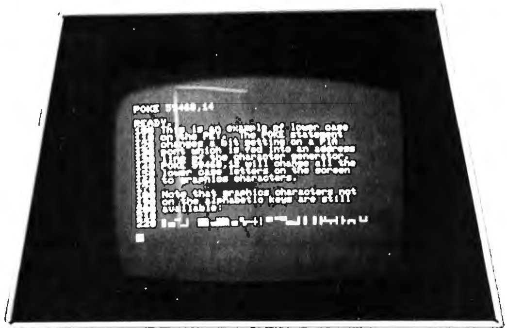
Photo 4: An illustration of upper and lower case letters on the PET. 26 of the 64 graphics characters can be exchanged for lower case letters by altering an address line on the character generator read only memory.
