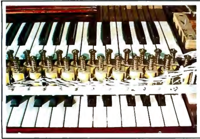
Photo 2: A set of solenoids used to automatically play the keys. Since this setup plays the keys directly, it could be easily adapted to any standard keyboard instrument including harpsichord and piano.
