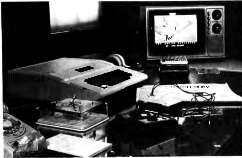
Photo 2: The Apple II in a typical use setting. The television is fairly far away from the computer itself in order to minimize interference and hash generated by the logic circuitry. An inexpensive cassette recorder with turns counter is used to provide mass storage for programs.
