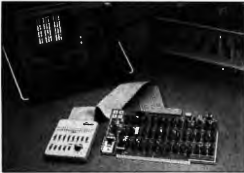
The Model 150 "Bus Grabber" logic analyzer electrically and mechanically
