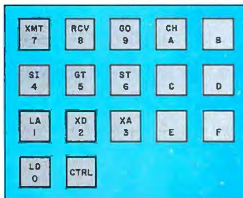
Figure 4: Detail of a microstation keypad. The normal mode of operation is hexadecimal input; when the CTRL key is followed by any other key, one of the 11 special functions (see text) is performed.
