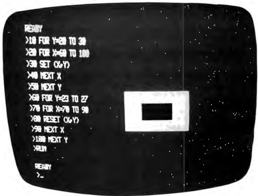
Photo 4: An illustration of the use of the TRS-80's graphics capabilities. The BASIC program shown on the screen created the square and cutout by using the SET and RESET statements to turn points on and off. This illustrates the arbitrary way in which text and graphics can be interspersed on the display.
