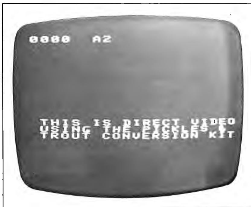
Photo 6: The same display source as that of photo 1, produced on the same TV set, but with the aid of the Pickles and Trout TVM-04. Note the sharpness of this direct video display in contrast to the RF entry of photo 1.
