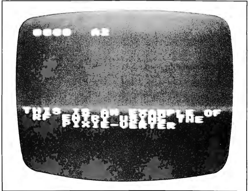
Photo 1: This display, produced by an ATV Research Pixe-Verter driven by an Ohio Scientific Instruments Model 440B video board, illustrates the RF modulator method of adapting an ordinary TV set to serve as a video monitor. This method requires no modifications to the TV set, but limits the number of characters that can be displayed on one line.
