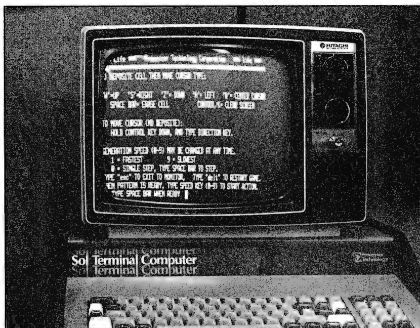
Photo 7: To illustrate the wider field possible with the Pickles and Trout direct video conversion, the 64 character display of a SOL-20 was used with the converted television perched on top of the SOL. We made no attempt to adjust the controls of the television set to remove the overscan condition evident in this photo of the Processor Technology LIFE demonstration program's output.
