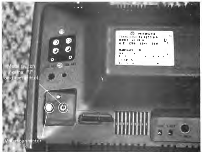
Photo 4: The TVM-04 lines up with the back of the TV set's plastic cabinet, giving access to a shielded cable connector for the video signal and a switch for selecting either normal program viewing or the computer generated display.
