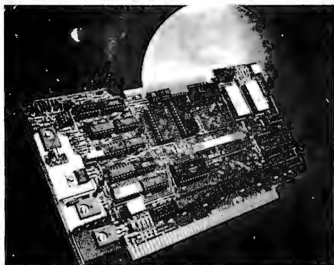
Infinite Incorporated, 1924 Waverly Pl, Melbourne FL 32901, has announced the MFIO-1, an Altair (S-100) compatible general purpose IO board. The
