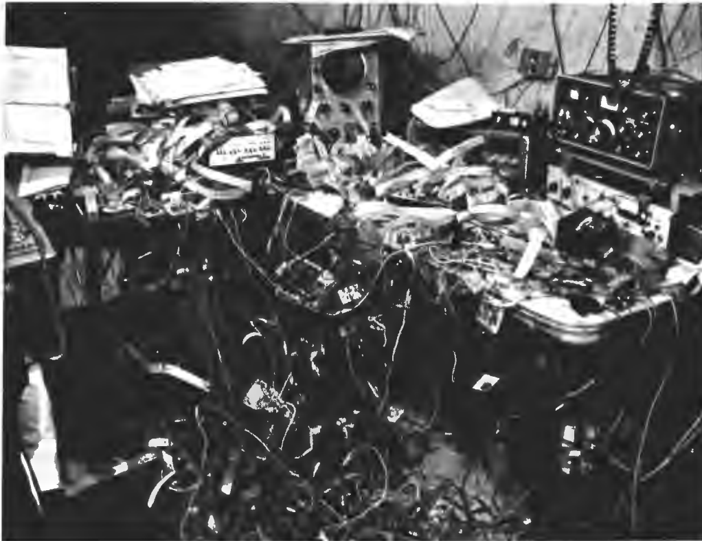
Photo 4: Roger Amidon's 4 bit processor, built in 1972 and fondly referred to as the "Spider." It was built with TTL logic and used to control an amateur radio (RTTY). The Spider was featured on the cover of April 1977 BYTE.
