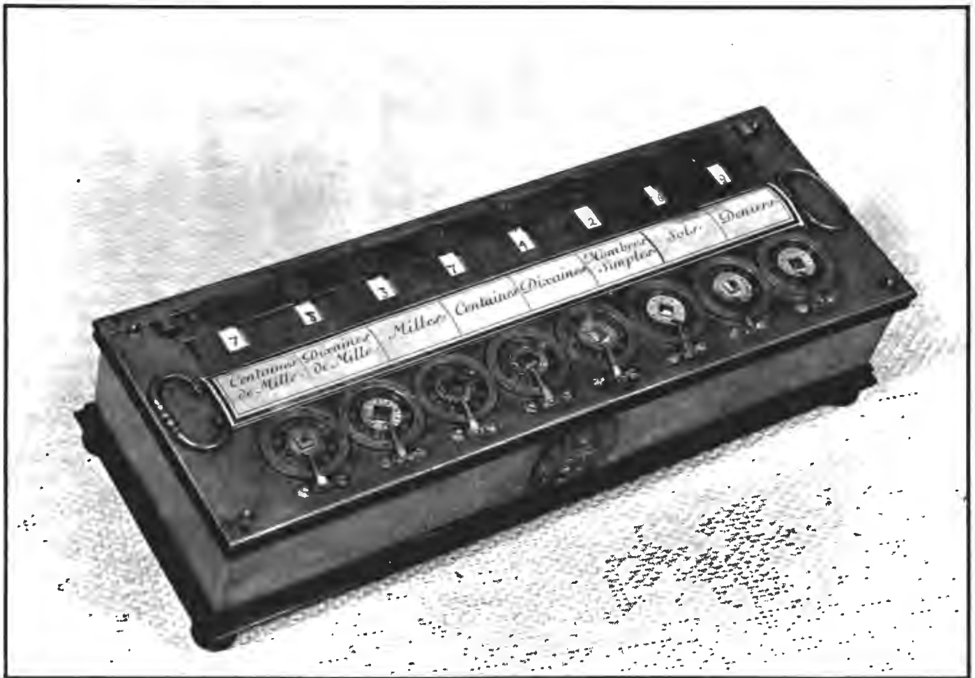
Photo 2: Pascal's adding machine. Note that the rightmost dial has 12 positions and its neighbor has 20. The machine was intended for calculations involving the French currency of the period.
