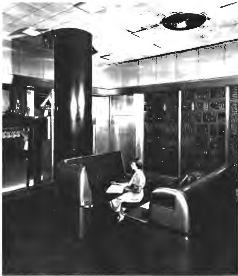
Photo 8: The IBM 704 had a core memory capacity of 32 K words with 36 bits per word. Although a card reader, punch, printer, magnetic tape drives and drums and a video display were available as peripherals, the concept of simultaneous IO and processing was not yet developed.
