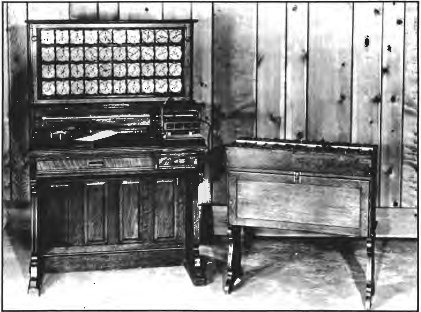
Photo 5: The first use of punched cards for data processing, Hollerith's card sorter dramatically reduced the time required to process data collected in the 1890 census.
