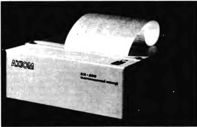
Photo 1: The Axiom EX800 printer. It uses special aluminized paper; when a tiny electrical spark jumps from the print head to the paper, the layer of aluminum is burned off revealing the next layer which is darkly colored. Printing speed is a maximum of 160 characters per second including upper and lower case letters. The printer allows 80 column page width and quadruple width characters.
