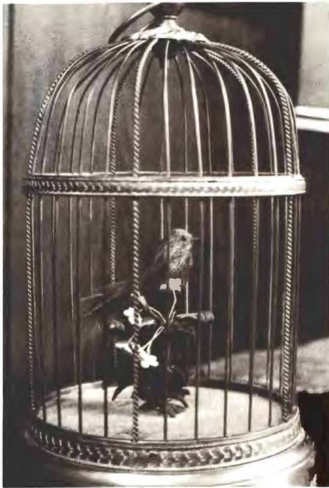
Photo 1: The bird organ, a popular novelty of the 18th and 19th centuries. The device is a sophisticated automaton capable of imitating the sound and movements of a real bird: the wings flap, the head turns, and the beak moves to the accompaniment of assorted bird whistles.
