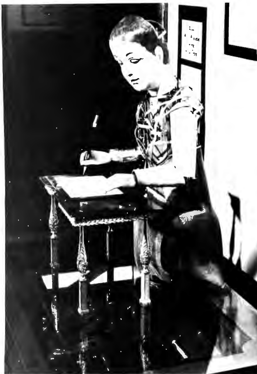
Photo 3: The Maillardet writing and drawing automaton sans clothes. The body of the figure is made from strips of brass and wire; the glass floor reveals the mechanism. A modern pen is shown in the automaton's hand. Courtesy Franklin Institute.
