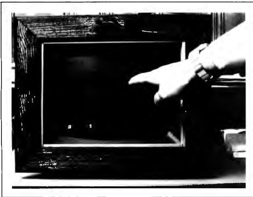
Photo 1: The basic information returned from the touch panel is a coordinate pair for one of 256 possible finger sized locations on the video display's face. Here, using the program in listing 3, the displayed coordinates 10 and 9 correspond to the point just touched on the screen.
