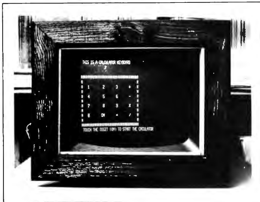
Photo 2: Here is a picture of an experiment which was backed up by a fairly long BASIC program: using the screen as the input device for a simulation of an ordinary 4 function calculator. The imagination of the user, to use a well-worn cliché, is the only limitation upon trying experiments with special purpose keyboards and interactive sequences on the screen. Use of the video display behind the touch panel area makes easily altered software the determining factor — rather than physical tools in the workshop.
