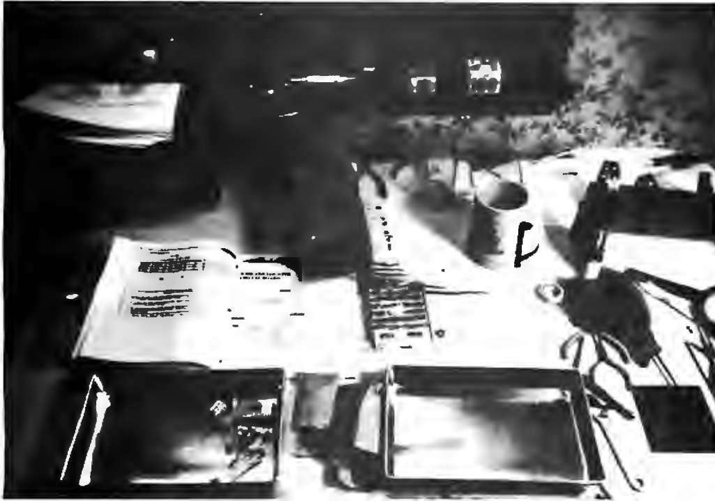
Photo 7a: A good practice when assembling complicated kits is built into the Heathkit manuals: a parts check off. In this photograph, the parts for the "RAM and counter circuit board" have been unpacked from the paper bags, with loose parts placed in the baking pan at the left.
