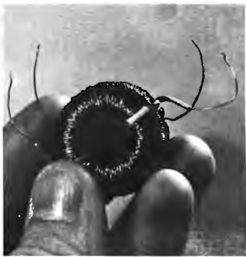
Photo 2: Surplus 88 millihenry toroidal transformer rewound with two secondaries of 175 turns of #26 wire each (after first unwinding the existing two windings of approximately 350 turns each). The unit is used in the circuit of figure 5a.
