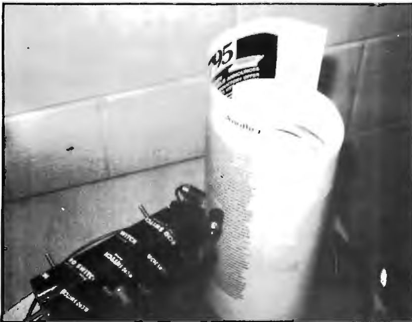
Photo 1: The authors' bar code reader entry. The page of bar code is shown taped to a fruit juice can sitting on a phonograph turntable. The reading arm, shown at bottom left, features two small lamps and a focusing lens. Light reflected from the rotating bar code energizes a phototransistor at the other end of the reading arm. The signal is then translated into binary voltage levels and sent to the computer's input port.
