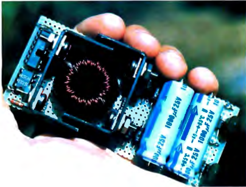
Photo 1: 5 W DC to DC converter, which produces 0.2 A at +12 and -12 VDC from a 5 VDC source. The circuit uses a special custom wound toroidal transformer (see figures 5a and 5b). Note: the prototype shown uses 1000 \mu F 25 V capacitors, which were later replaced with 100 \mu F 25 V versions.
