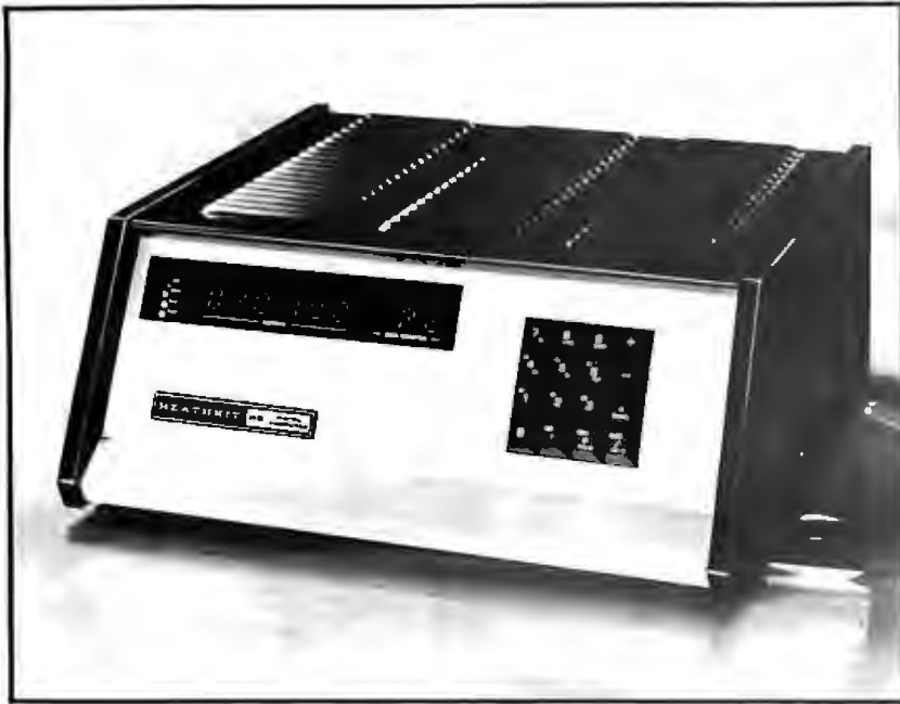
Photo 1: Front panel of the Heath H8 computer. At left are nine 7 segment LED displays and four single LED lamps; at right is the 16 key keypad. The front panel is controlled by a novel firmware panel monitor (PAM/8) made up of both hardware and software elements.
