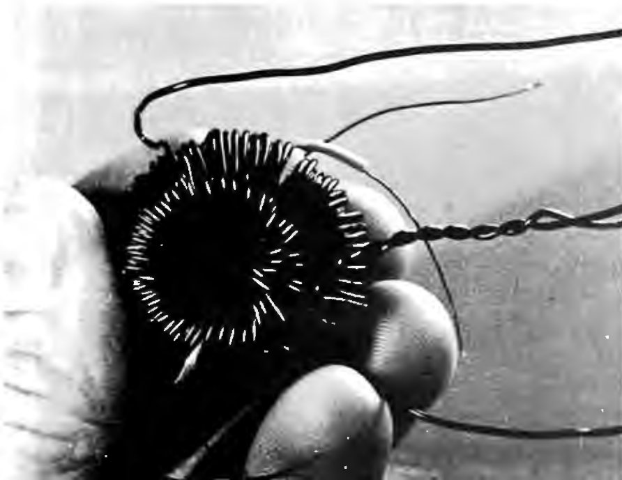
Photo 5: The completed transformer. The ends of all enameled wires should be cleaned of insulation before soldering.
