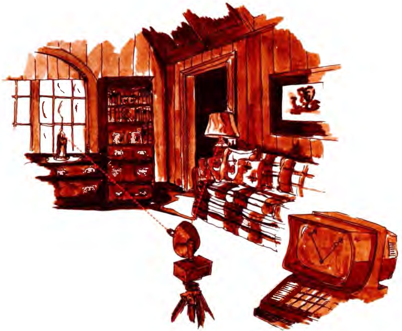
Circuit Cellar experimental setup showing the parabolic scanner as it detects a candle.
