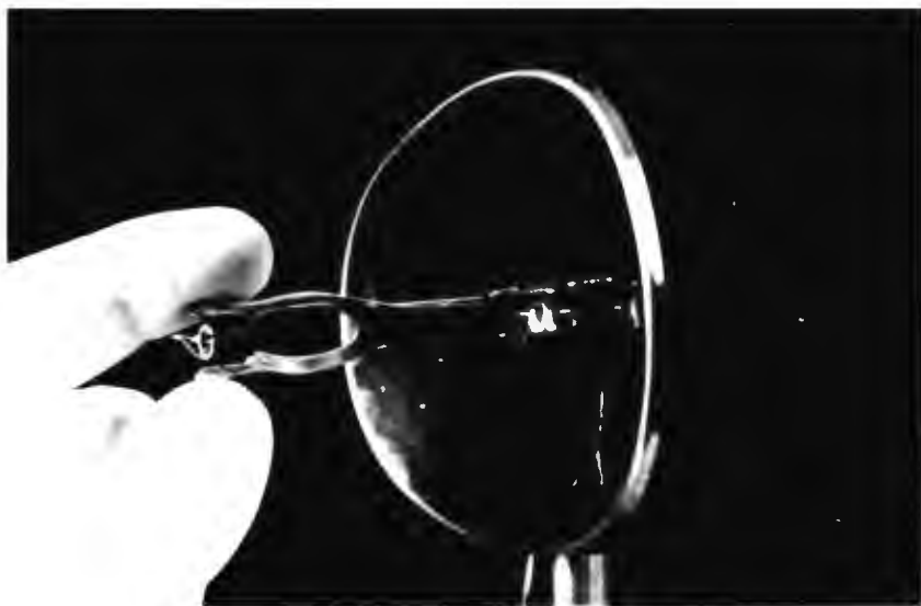
Photo 2: The parabolic reflector, used to gather light for detection by the photo detector.
