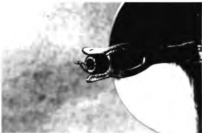
Photo 3: Closeup of the photo detector glued to the pronged holder.
