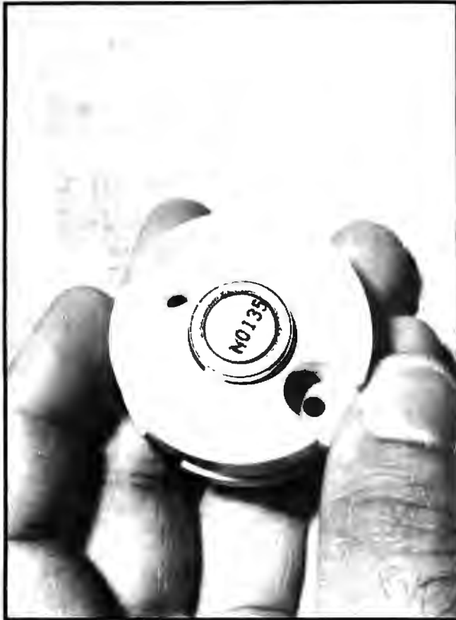
Photo 3: Heat sensor designed to trip above 135° F, typical of the type often used in combination with smoke detectors.
