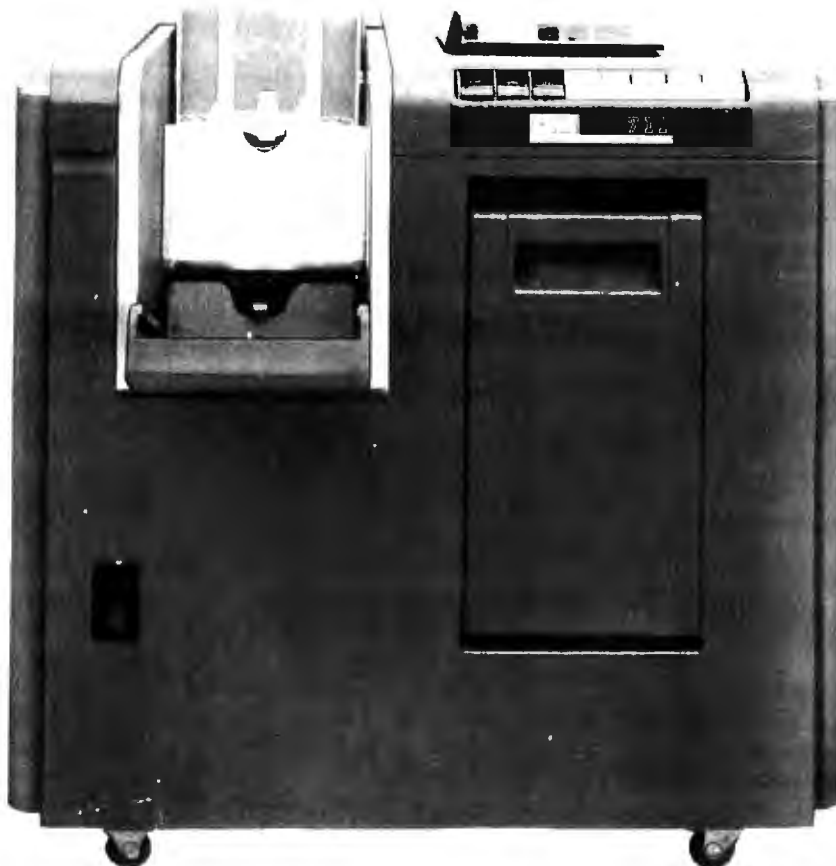
Photo 3: The 711 on line card reader read 24 36-bit numbers in row binary format from columns 1 thru 72. Columns 73 thru 80 could not be read.
