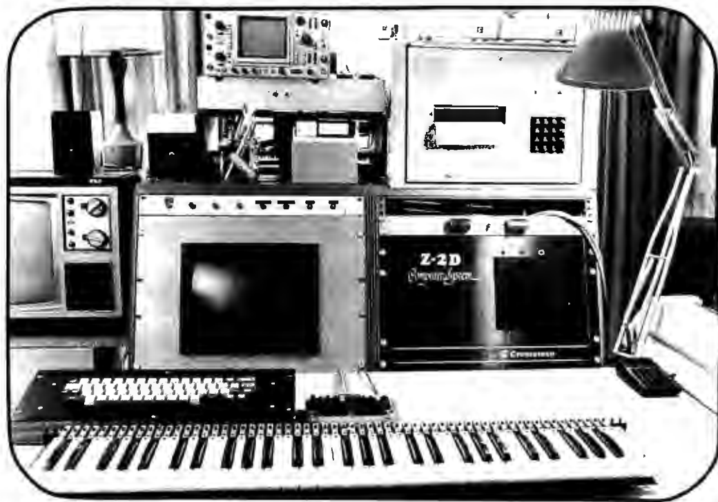
Photo 1: The author's polyphonic music keyboard system, which allows more than one note to be played simultaneously. The scanning keyboard interface is just behind the 61 note manual in the foreground. The stand alone ASCII keyboard in front is dedicated to music related tasks, and, in conjunction with a video terminal (not shown), allows two easily distinguished levels of system control.
