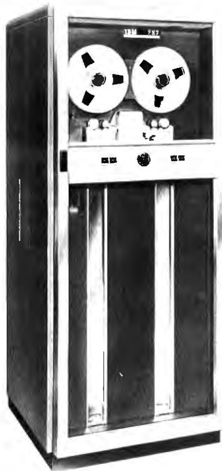
Photo 4: The 727 tape drive, over 20 years old, is similar in appearance to modern tape units. Note the address selector dial between the two rows of buttons.
