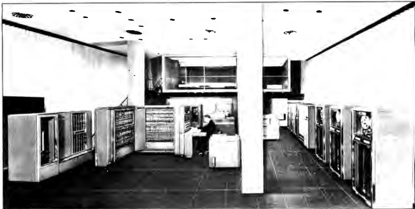
Photo 1: The IBM 704 data processing system. Along the left wall of the room is the magnetic core storage. The operator's console is in front of the central processing unit. Along the back wall is the power supply, printer, card reader and card punch. The magnetic tape units are lined up along the right side of the room.
