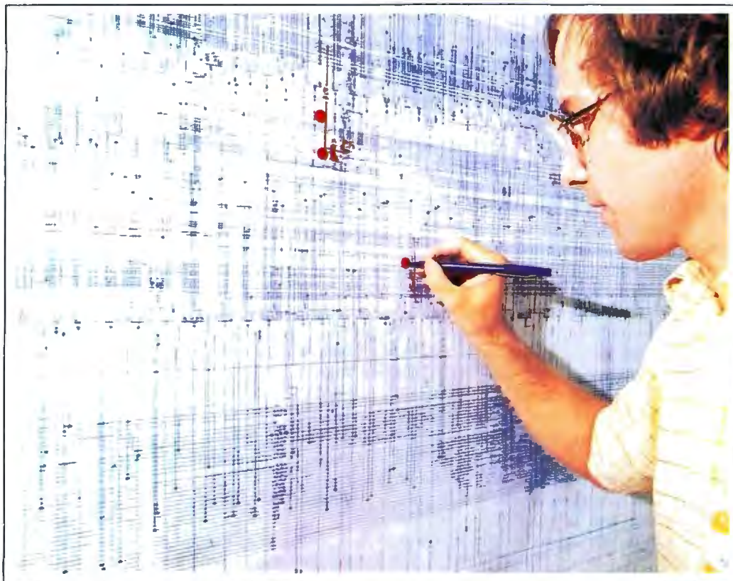
Photo 2: Breadboard design. After partitioning the logic, the MOS (metal oxide semiconductor) diagram is translated to TTL. The required ten boards are then designed and built. Meanwhile, Bill Keshlear updates the logic changes on the master copy of the logic diagrams, since they will imply changes on the boards.
