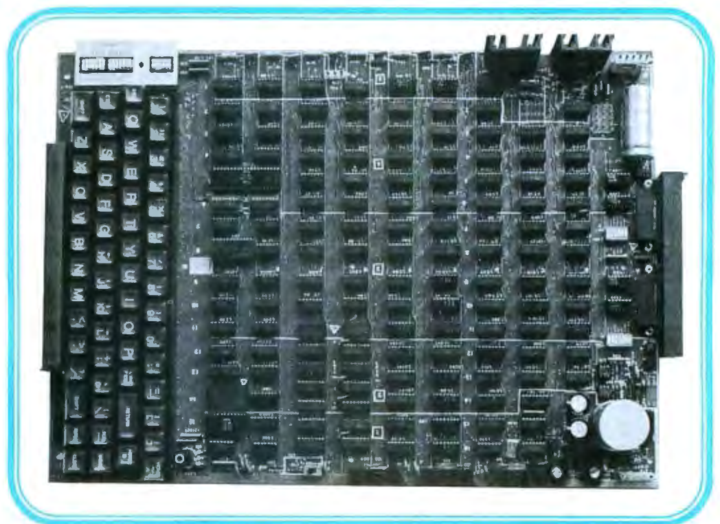
Photo 2: Most of the circuitry is assembled on the large printed circuit board shown. This includes the keyboard and power supply.
