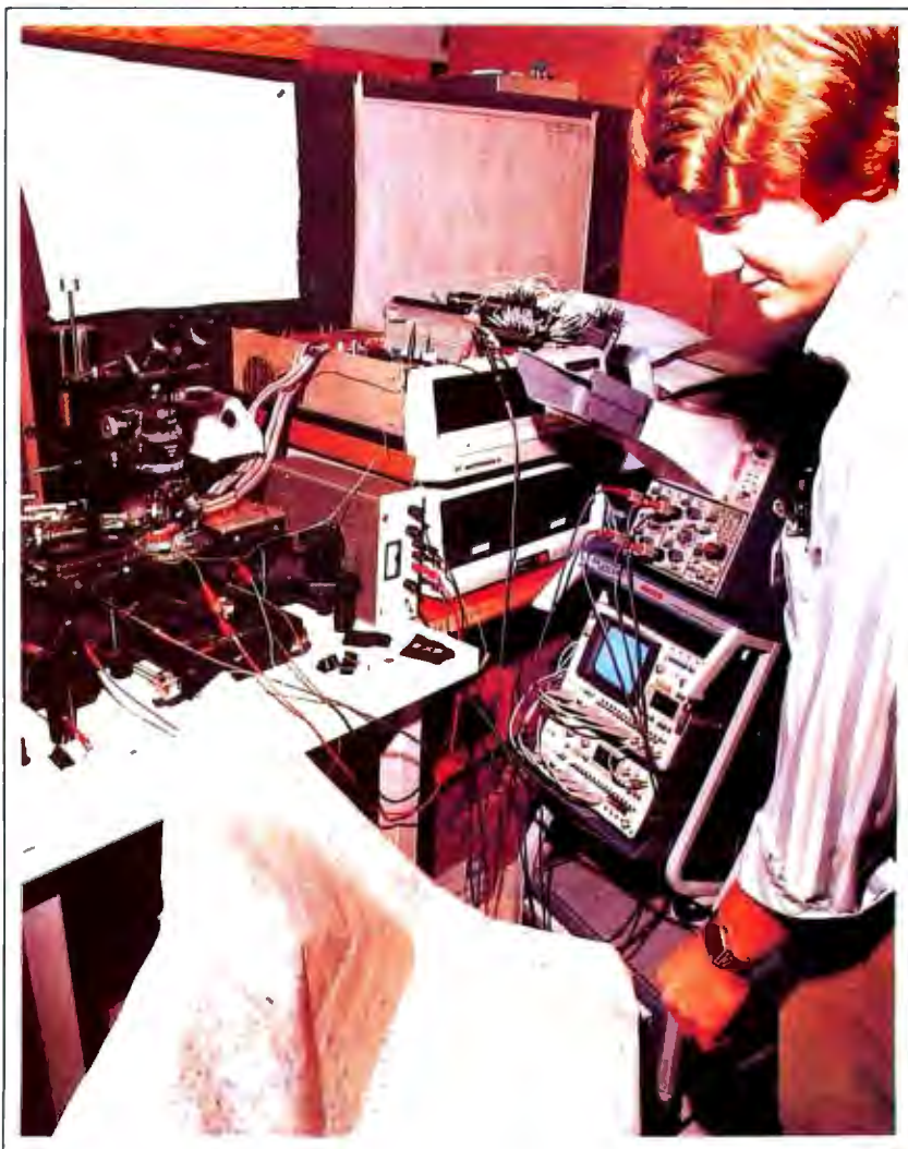
Photo 5: First silicon engineering analysis. Logic and circuit design engineer Bob Thompson tracks down a weak node in the first batch of 6801 chips. The 6801 die is packaged, but not sealed, so that internal nodes may be probed while in operation. Viewing through the microscope, a probe can be placed at critical points equivalent to the layout plot. The chip itself is running a modified EXORcisor system, and the scope actually displayed an internal signal with excessively slow rise time.
