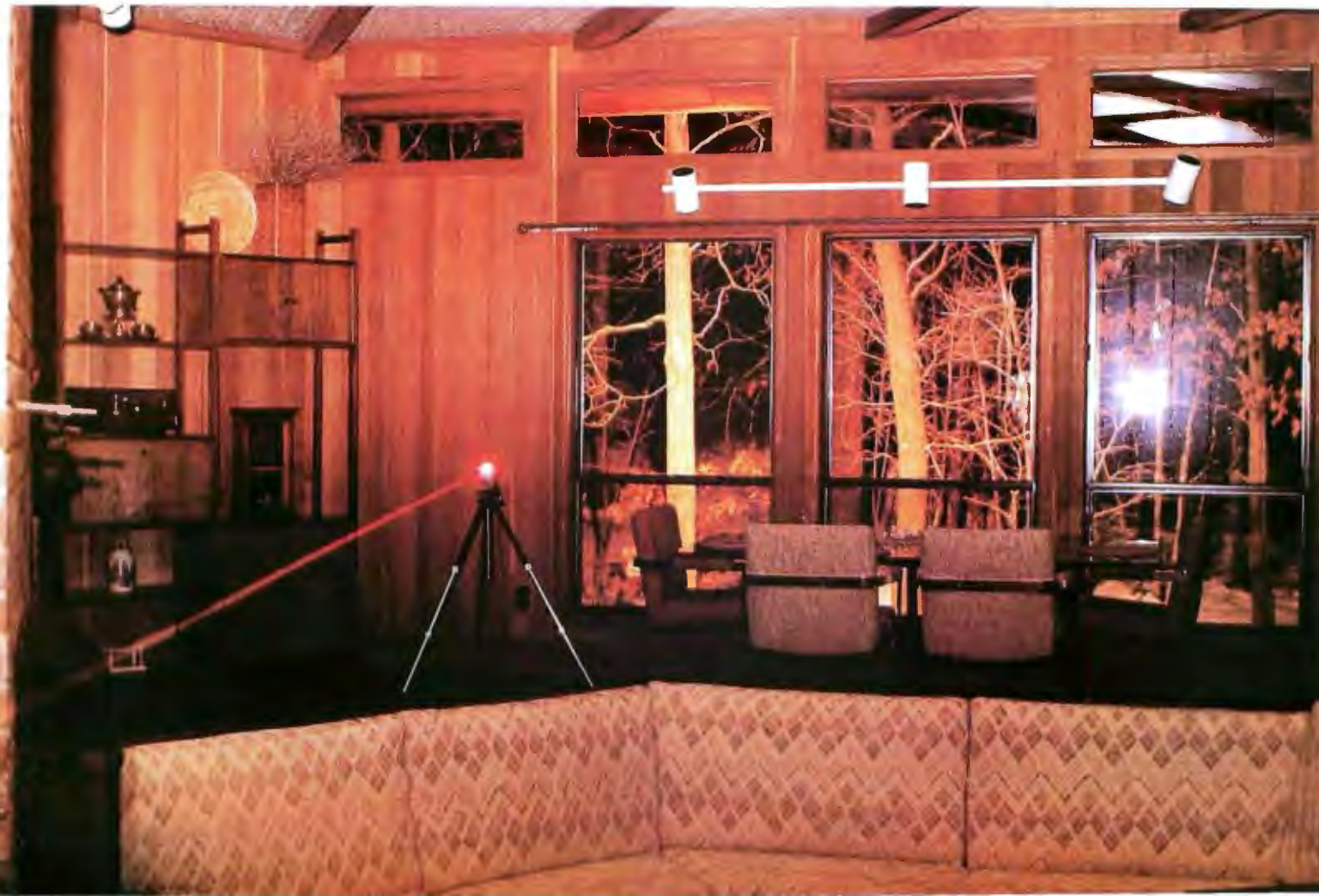
Photo 3: A laser on a tripod shooting across my living room. The laser is a 2.2 mW unit built by Metrologic Instruments of Bellmawr NJ 08031 (this particular model is the ML-969). This picture was taken at night; the trees outside are illuminated by outside flood lamps.
