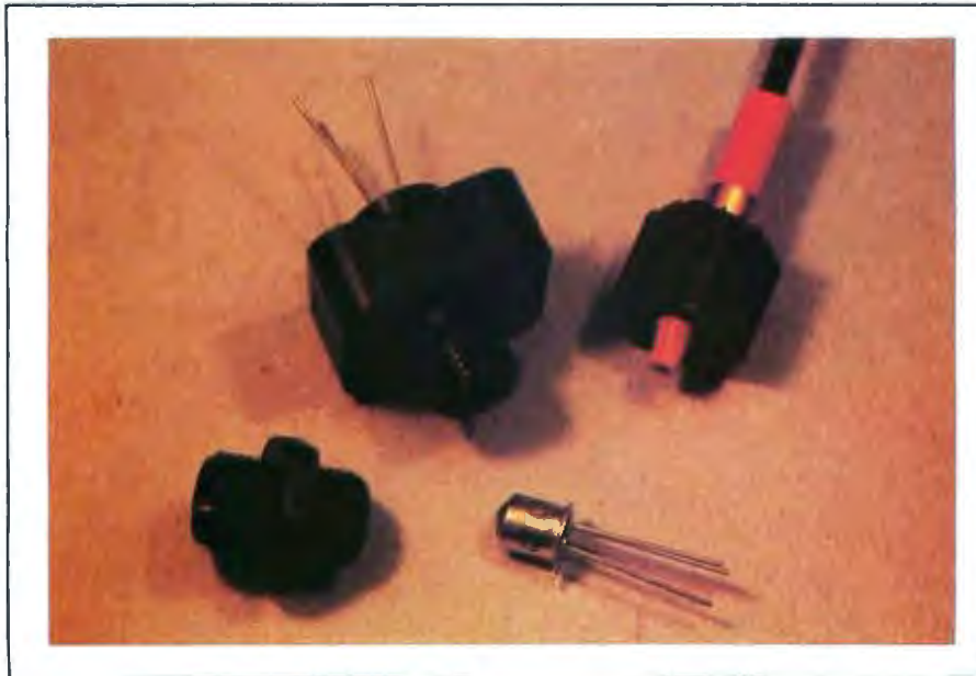
Photo 2: Special connectors necessary to use fiber optics properly. Shown here (starting in the upper right corner and continuing clockwise) are a fiber optic cable with an end connector, a phototransistor in a TO-18 package, an extension coupling which allows two cables to be connected, and a bulkhead receptacle containing either an LED (light emitting diode) or phototransistor.
