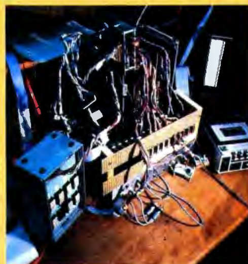
Photo 1: This homebrew personal computer system is an example of the kind of packaging nightmare which can result from experimentation with hardware. It works quite nicely, but is not exactly portable. This system proves that in hardware, as in software, it is possible to get a system where the patches and ad hoc kluges tend to outnumber the original features of the design.
