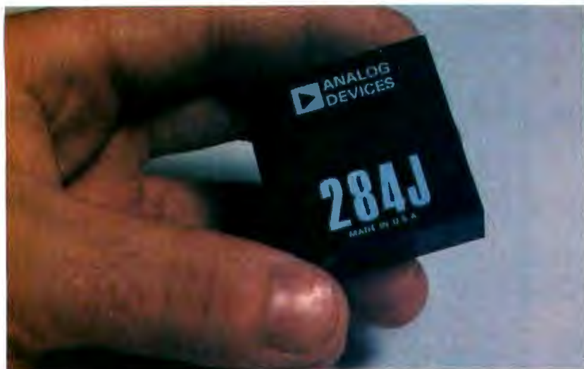
Photo 2: The Analog Devices 284J isolation amplifier used in this article.
