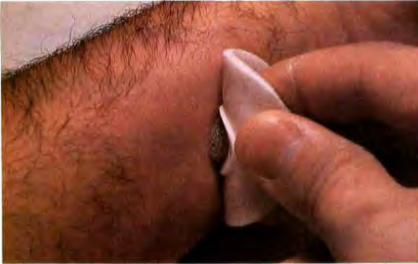
Photo 5: The electrode has a saturated spongy center which serves to reduce skin contact resistance. It is necessary to use this type of connection to the body if satisfactory results are to be obtained.
