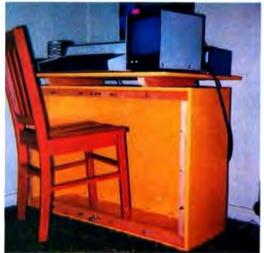
Photo 2: The system as it appears when converted into a desk. Note that the floor of the cabinet becomes a desk top displaying the entire system ready to plug in and run.
