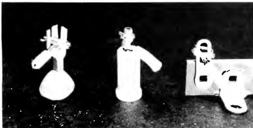
Photo 2: Before soldering, the joints should be mechanically fastened.
