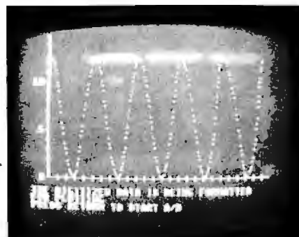
Photo 1: High-resolution display of a 0.05 Hz sine wave signal which has been digitized at 10 samples per second.
