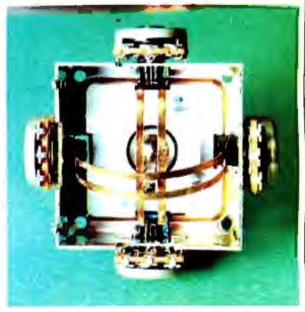
Photo 2: Note how moving the stick moves the gimbal arrangement, which in turn changes the settings of the potentiometers.
