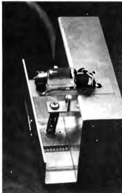
Photo 1: View of the paper-tape reader showing the light source and the light-detecting phototransistors. The spring and clamp device keeps the paper tape in place.
