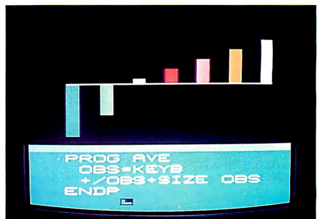
Photo 2: Program AVE, which computes the average of a set of numeric observations. Input is from the keyboard as a series of numeric values — an array constant. The input, returned by the KEYB function, is assigned to OBS, thus making OBS an array. The average value is computed by adding up the elements of the array (+/OBS) and dividing the sum by the size of the array (SIZE OBS). Since the result is not assigned to a variable, it is displayed.
