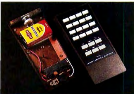
Photo 4: Handheld cordless controller showing top and internal circuitry.
