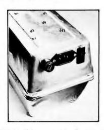
Photo 2: Holes were cut to allow mounting of a fuse, a 3-prong connector, and a switch (with an internal neon pilot lamp).
