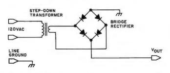
Figure 2: Schematic diagram of the power supply without capacitor or regulator. This circuit produces the output voltage waveform shown in figure 3.
