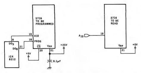
Figure 5: Modifications to the circuit of figure 3 that enable the programming of the 2716-type EPROM. Modifications to the software are also necessary.
