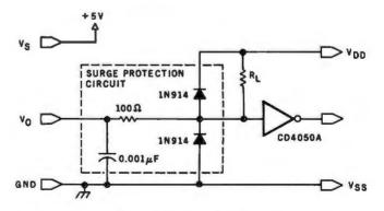
Figure 1: A pair of schematics showing (1a) the TTL interface for the HEDS-3000 bar-code reader, and (1b) the CMOS-logic interface. This diagram is reproduced from page 9 of the HEDS-3000 Digital Wand User's Manual, which accompanies the reader in a prototyping kit.
