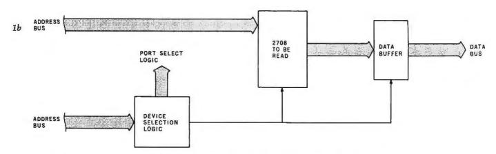
Figure 1: Block diagrams of the 2708 EPROM programming circuit (1a) and 2708 reading circuit (1b).
