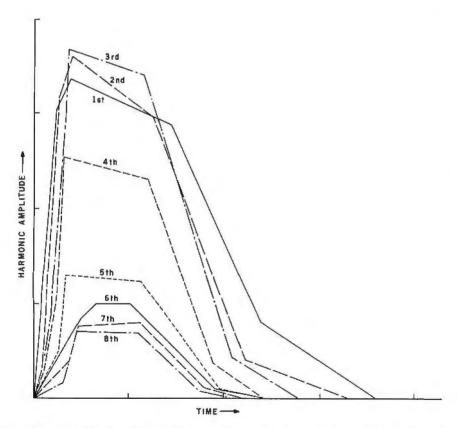
Figure 7b: Simplified analysis of a trumpet note. The complex curves seen in figure 7a have been divided into relatively long line segments to reduce the amount of information necessary to specify the sound to the computer. The graph here is based on Moorer's straight-line-segment simplification of his trumpet analysis; see reference 3.
