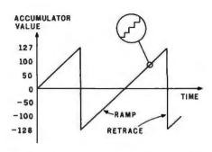
Figure 1: Generation of a sawtooth waveform by software. Coordinate points along the waveform are generated by continuously adding a constant value, FREQ, to the accumulator (register A). The point values (samples) are sent to the D/A converter. A close-up circle demonstrates the inevitable stair-step quality of the curve reproduced from discrete samples. The 6502 assembler code to produce the sawtooth is shown in listing 1.
