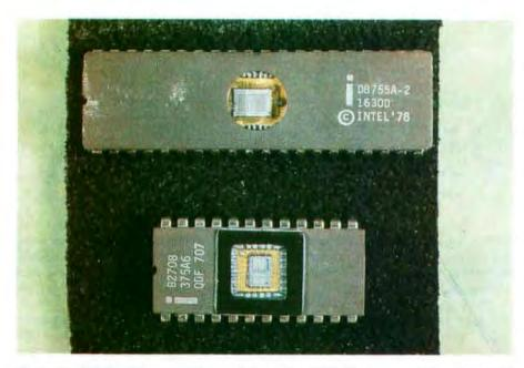
**Photo 2:** Side-by-side comparison of the 8755 EPROM, top, and the older 2708 EPROM. The difference in package size is due to the presence of I/O ports on the 8755. The 8755 requires a single 5-V power supply and contains 2 K bytes of memory; the 2708 requires three different power supply voltages (+5 V, +12 V, and -12 V) and contains 1 K bytes of EPROM.
