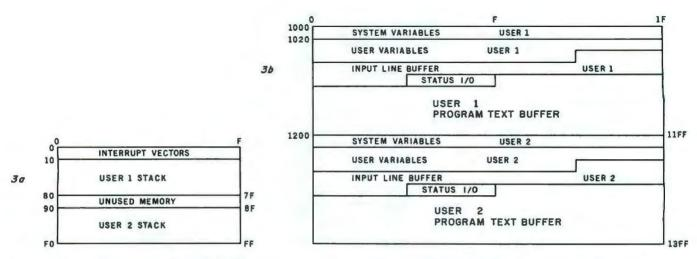
Figure 3: Map of memory use of the 8088 multi-user operating system. Programmable memory from hexadecimal addresses 00 thru FF is contained in the 8155 integrated circuit and is used chiefly to hold the pushdown stack for each user. Memory from hexadecimal locations 1000 thru 13FF is in the 8185 device, and stores various data belonging to the two user-tasks. Memory from hexadecimal addresses 0F800 to 0FFFF takes the form of EPROM in the 8755A, which stores the operating system,
