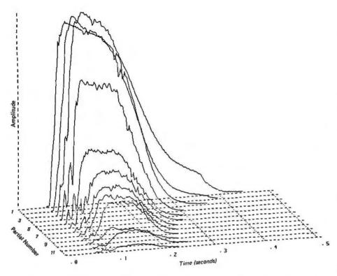
Figure 7a: Computer analysis of a tone produced by a trumpet. This is a two-dimensional projection of a three-dimensional plot. Amplitudes of different harmonics present in the note have different attack and decay characteristics. (Figure reproduced from the Computer Music Journal, volume 2, number 2, 1978, page 1; used by permission).
