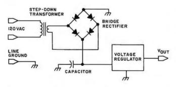
Figure 1: Schematic diagram of a typical power supply circuit containing a step-down transformer, a full-wave bridge rectifier, a filter capacitor, and an integrated circuit voltage regulator.
