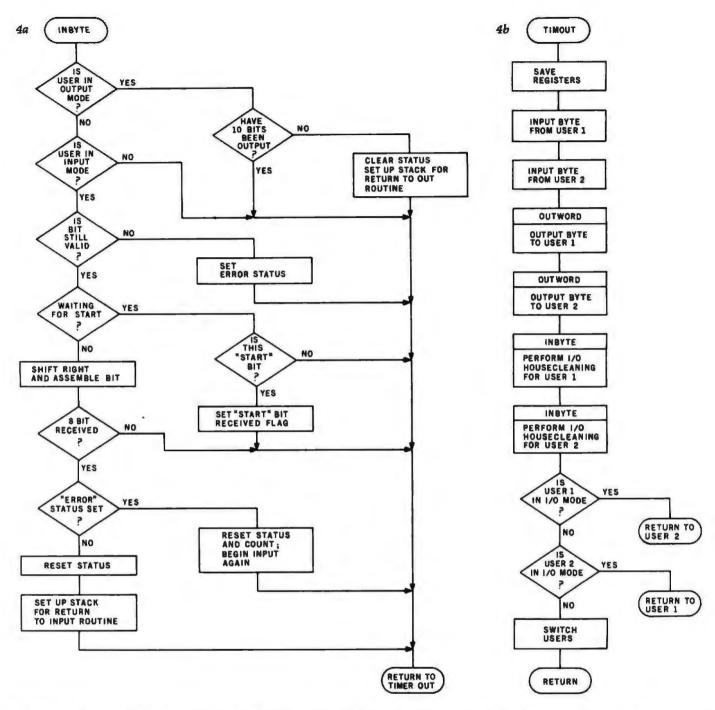
Figure 4: Flowchart of the multitasking routine of listing 1, which divides the resources of the 8088 system between the two users.
