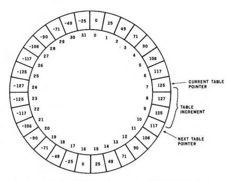
Figure 4: Conceptual diagram of a waveform-scanning table. The table, in this case containing thirty-two waveform samples, is scanned in such a manner that the end of the table seems to be contiguous with the beginning. The table pointer indicates the value that is currently being sent to the D/A converter. During each sample period, a tableincrement value is added to the table-pointer value, vielding a new pointer position further around the table.
