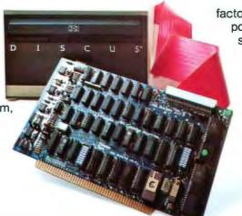
factory mounted in a cabinet with power supply, fully-buffered S-100 single-board controller, and interconnecting cables. All fully assembled, system-tested and fully warranteed. You get the speed and efficiency of 1.2 megabyteper-diskette memory... and you get it for 0.13¢ per byte.
