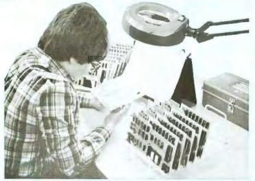
"Slipping a circuit board through the eye of a needle would be easier than slipping a cold solder joint past Beverly. These are four-drive LFD-400/800 disk system controllers she's inspecting."
