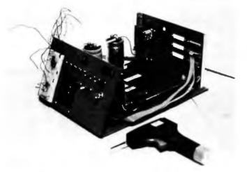
Photo 1: The author's homebrew COSMAC computer system. It contains 2560 bytes of memory and uses a full 16-bit address display. Important processor and input/output signals are brought out through the front panel for ease in breadboarding.
