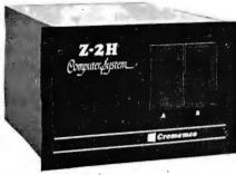
• Full 11-megabyte hard disk system • fast Z80A 4 MHz processor • two floppy disk drives • 64K RAM memory • BS232 special interface • printer interface • extensive software available
