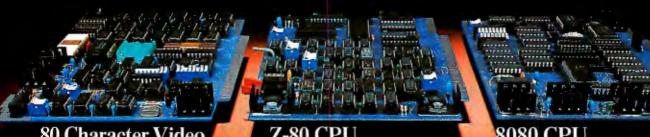
With 80 characters per line our VB3 is the perfect video interface for processing. It produces a standard 80x24 display of upper and lower case characters or as much as 80x51 for a full page of text. The matrix for graphic display goes up to 160x204. And with optional EPROM, as many as 256 user programmed characters or symbols can be produced.
