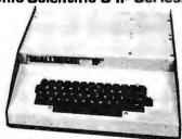
The Challenger 1P. The best bargain in personal computer anywhere! BK BASIC-in-ROM. 4K RAM. Cassette based with 53-key keyboard. B&W video interface, 30 rows x 30 columns. Upper and lower case.
