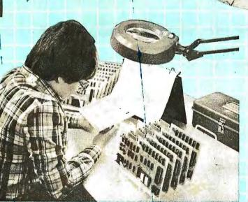
"Slipping a circuit board through the eye of a needle would be easier than slipping a cold solder joint past Beverly. These are four-drive LFD-400/800 disk system controllers she's inspecting."
