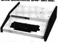
The Challenger 4P. A 4-slot computer with one open slot. Highly sophisticated 16 color video interface. 32 rows x 64 columns, upper and lower case. BK BASIC-in-ROM, BK RAM. 200-20KHz programmable tone generator. AC remote interface. Expandable to 32K RAM and two mini-floppy drives. \$750.
