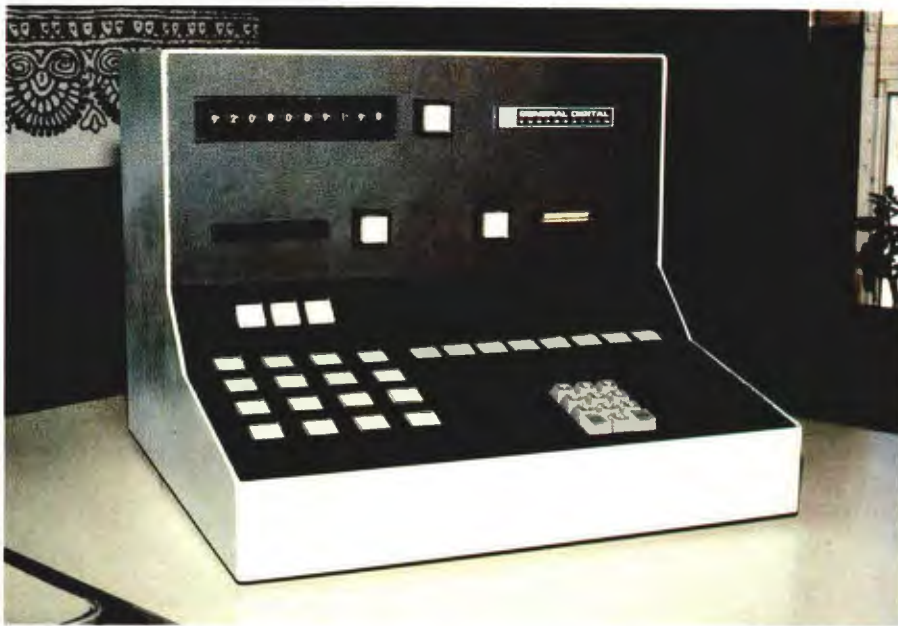
Photo 1: Deluxe remote data-entry terminals, intended for industrial use, often contain specialized equipment to read card-badges, or control unusual functions. Many are constructed with a hazardous environment in mind, and are waterproof or blast-proof. This particular unit is a function/numeric panel (FNP) manufactured by General Digital Corporation in East Hartford CT.
