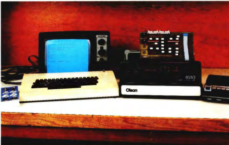
Photo 1: A wolf in sheep's clothing. The panel may say "8080," but the processor card in this system is based on Intel's high-performance 8088.
