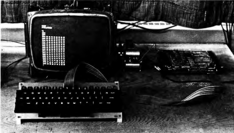
Photo 6: The complete terminal system with keyboard, monitor, power supply, and main circuitry.
