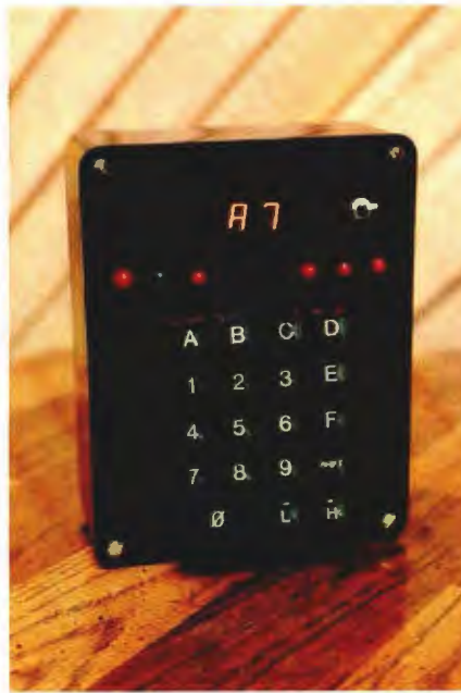
Photo 2: The remote data-entry terminal. Using a new serial keyboard-interface integrated circuit, construction is simple and inexpensive.
