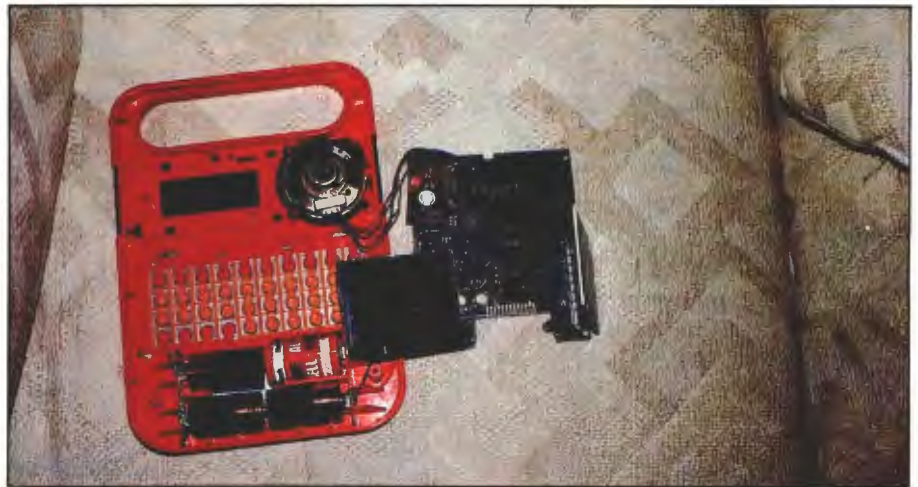
Photo 1: Detailed photograph of the disassembled Speak & Spell. The main circuit board is shown in the same position as in figure 2; the board in the upper left-hand corner is the power supply. The black box at bottom center is one of the two keyboard assemblies.
