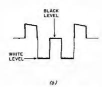
Figure 8: Sample video display and corresponding composite video signal. The low portion of the composite signal (b) turns on the electron beam to illuminate the screen (a). When the intermediate voltage of the black portion is encountered, the beam is turned off. As the composite signal returns to the low white level, the screen is illuminated again.
