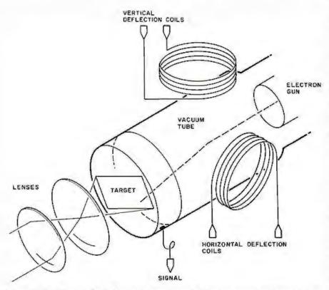
Figure 2: A vidicon tube. This most popular method of converting an image into an electronic signal uses a photo-sensitive imaging target which is scanned by an electron beam. The resulting signal is the scanned image in the form of a changing voltage. Disadvantages of the vidicon are its unstable geometry (since electron-beam deflection is never completely repeatable and accurate) and its low resistance to shock (since vidicons are vacuum tubes).
