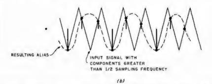
Figure 7b: If high-frequency components are present in the video signal which are above one-half the sampling rate, false information (aliasing) results. Aliasing is a beat frequency between the sampling frequency and those signal components above one-half the sampling frequency. A low-pass filter is used to filter the frequency components and eliminate aliasing.
