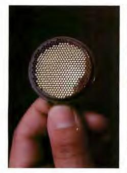
Photo 3: Close-up view of the Polaroid Ultrasonic Transducer.
