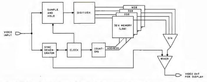
Figure 10: Block diagram of an image-quantization system. In this example, a single memory board is used for each bit of quantization. Four boards would be needed for a 4-bit quantization.
