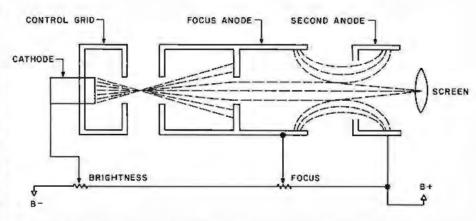
Figure 3: Focusing the beam. By applying the proper potentials to the anodes and control grids, the electron beam can be "squeezed" to a pinpoint, for displaying the image on the screen.
