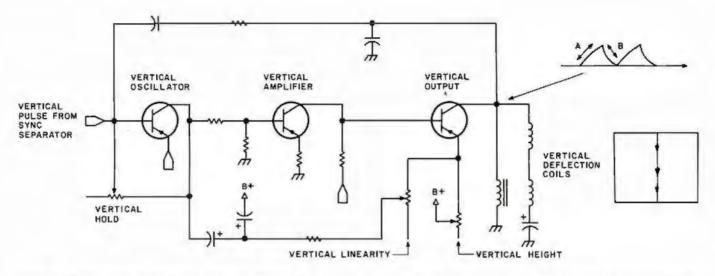
Figure 4: Typical vertical oscillator/amplifier section. The circuitry shown creates a sawtooth waveform to drive the vertical deflection coils. This enables the electron beam to move from the top of the screen to the bottom 60 times per second.
