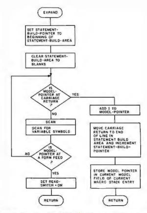
Figure 9: Flowchart for EXPAND subroutine. This subroutine expands a model statement using the current values of the variable symbols as found on top of the symbol table.
