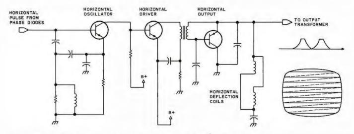
Figure 5: Typical horizontal oscillator and output yoke. The horizontal deflection coils are driven in a manner similar to the vertical deflection coils, but at a much higher rate of 15,750 Hz.
