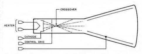
Figure 2: The crossover effect. Two accelerating anodes, in conjunction with the focusing anode, are used to give a sharp beam and a well-defined screen image. Without the focusing arrangement, the electron beam diverges and splatters.
