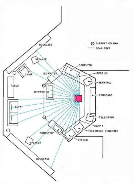
Figure 7b: Floor plan of Circuit Cellar showing location of scanner and beam paths to room objects during the twenty-five steps in the scanning sweep. Bar graph of figure 7a shows relative distance to the nearest obstruction in the beam path at each step.
