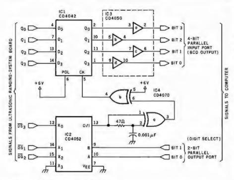
Figure 5: Schematic diagram of an interface that allows a computer to directly read the three-digit LED display of the EDB, using four integrated circuits. Through 2 bits of a parallel output port, the computer sends a digit-select code and then reads the corresponding BCD value of the selected digit through 4 bits of a parallel input port.
