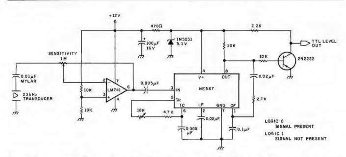
Figure 2: Ultrasonic receiver. This simple receiver has TTL-compatible outputs, and it will work with either transmitter in figure I.
