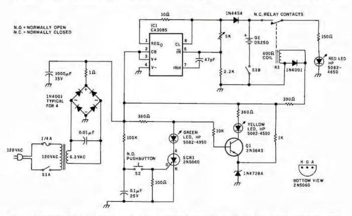
Figure 1: This power-line-failure indicator uses a silicon-controlled rectifier to detect voltage dropouts. If power should fail for more than 0.3 seconds, the SCR ceases to conduct and the green LED is extinguished, while the red LED lights. The red LED remains on as long as power is out; its power is drawn from a set of rechargeable batteries. Should power return, the red LED goes out and the yellow one is illuminated to indicate this sequence of events.
