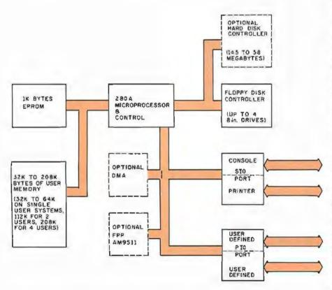
Figure 1: Block diagram of the Altos AC58000 systems.
