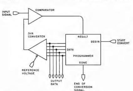
Figure 11: The configuration of a conventional A/D converter.
