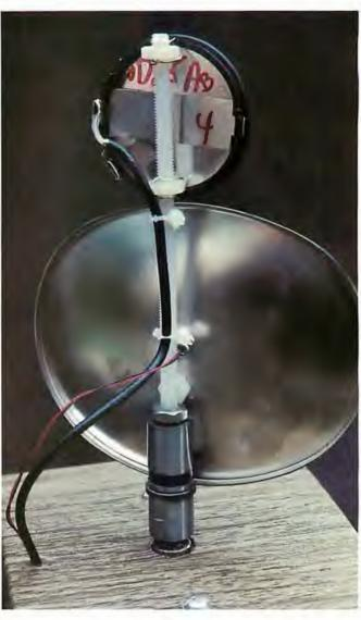
Photo 8: Close-up of the back side of the reflector and transducer of the scanner, showing the mounting apparatus.
