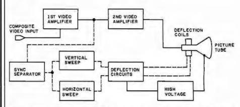
Figure 9: Block diagram of the signal path in a typical monitor. The solid lines represent actual video information, while the dashed lines indicate the path of synchronization signals.
