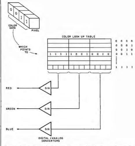
Figure 4: Color-look-up table. Using this scheme, a 4-bit value from the frame buffer (shown in figure 3) can select one of sixteen predefined colors. In this example, each color is composed of various intensities of red, green, and blue. Other systems may specify colors by indicating values for intensity, hue, and saturation.
