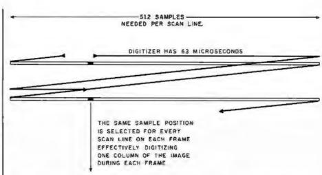
Figure 8: By sampling a single point per scan line, the digitization of each pixel can be completed within 63 µs, and data is produced at a slow enough rate (15.7 k bytes/second) for transfer to mass storage.
