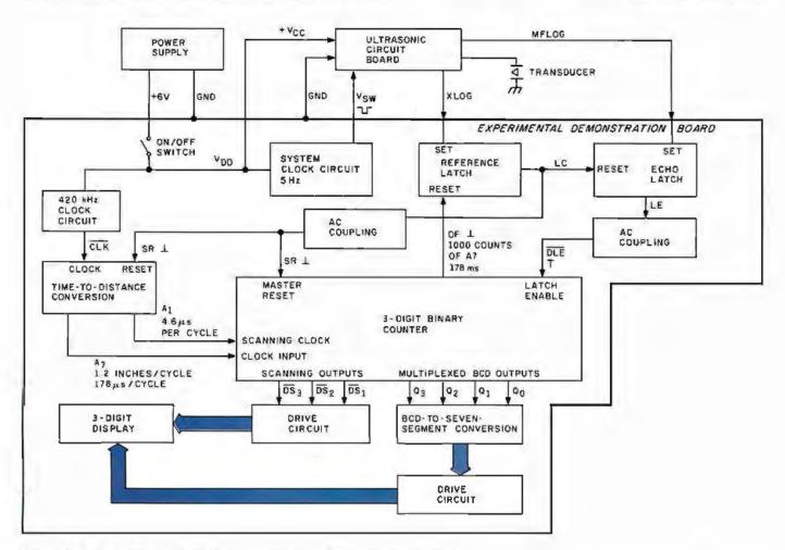
Figure 3: Block diagram of the Polaroid Experimental Demonstration Board.
