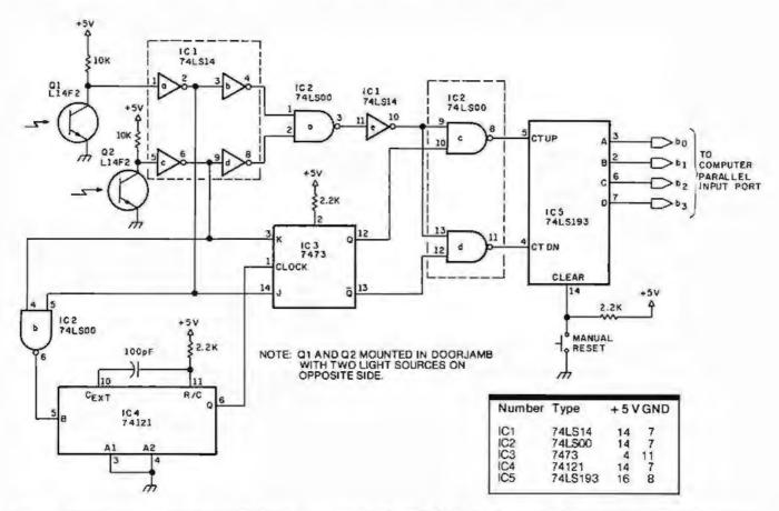
Figure 3: This circuit is capable of optically detecting the passage of people through a doorway and maintaining a count of people in a room. The photo-transistors sense motion through the doorway and cause the count stored in IC5 (a 4-bit binary counter) to either be incremented or decremented, depending upon the direction of passage.
