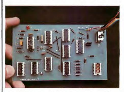
Photo 6: The EDB, which contains the electronic circuitry shown in figure 4. The three-digit LED display is at the upper right.
