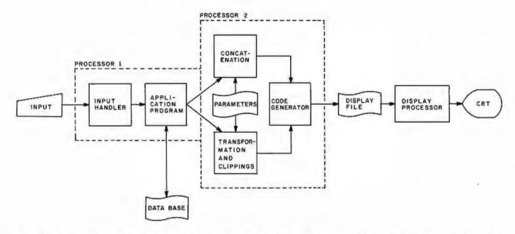
Figure 1: A general block diagram of an interactive graphics-display system. The functions of Processor 1 and Processor 2 may be performed by the same device; however, the output of Processor I must be a structured abstract of the image to be displayed, for the graphics package (Processor 2) to operate. (The figure is from Principles of Interactive Computer Graphics, by Newman and Sproull. Copyright 1973, used with permission of McGraw-Hill Book Company.)
