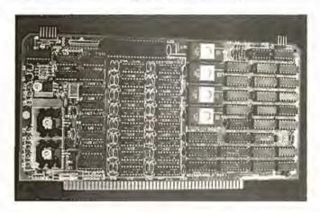
Photo 2: A close-up of the MicroAngelo S-100 board. The board has a Z80A microprocessor, 32 K bytes of memory, and four 2708 PROMS (expandable to 8 K bytes 2716 PROMS). The board is actually a stand-alone 32 K computer. The video display generates 512 by 480 dots. In the ALPHA mode, up to 85 by 40 characters may be displayed on the screen.
