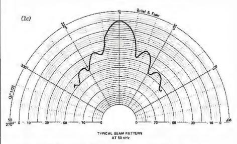
Figure 1: Typical transmission frequency-response curve (1a), reception frequency-response curve (1b), and radial-beam pattern (1c) of the Polaroid ultrasonic transducer. The beam pattern was measured at 50 kHz, with dB values normalized to on-axis response.
