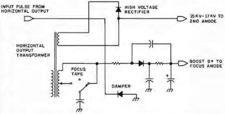
Figure 6: Typical high-voltage circuit. High-frequency AC from the horizontaldeflection circuitry is also used to produce the high voltage supplied to the focusing and second anodes. After passing through a step-up transformer, the AC is rectified and filtered for use in various other circuits.
