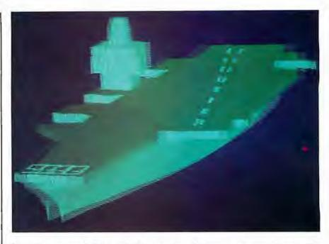
Photo 10: Interlaced left-eye and right-eye view of a computer-generated image of an aircraft carrier. The image is viewed in three dimensions when the user wears glasses with lenses made of PLZT (lead lanthanum zirconate titanate) ceramic. The lenses by the right and left are darkened alternately by voltage pulses synchronized to the display. Photo courtesy of John A Roese and Larry E McCleary, the Naval Ocean Systems Center.
