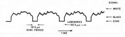
Figure 4: Each line of a video signal is composed of a horizontal active-line period (53.3  $\mu$ s), which contains the luminance information, and a sync period (10.2  $\mu$ s), which contains reference levels and the horizontal sync period.
