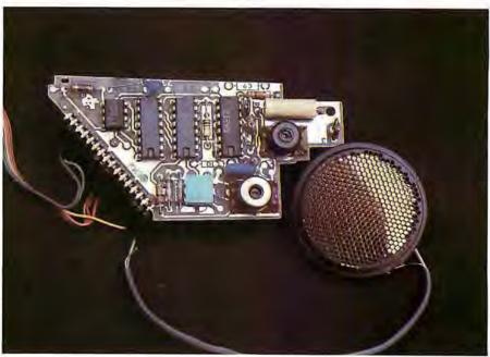
Photo 4: Close-up of the ultrasonic circuit board, which contains custom analog and digital integrated circuits.
