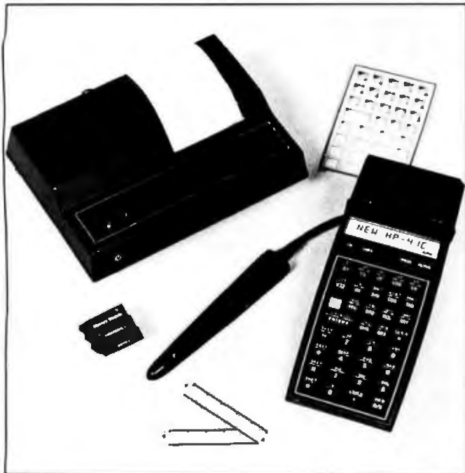
Photo 2: The HP-41C and accessories. Clockwise from top are: the 82143A peripheral printer, a key overlay (for use when redefining key functions), the HP-41C with the 82104A plug-in card reader, two magnetic cards, and three read-only-memory application packs. In the center is the 82153A bar-code wand, which is used to read software printed in the form of bar codes. (Photo courtesy of Hewlett-Packard.)
