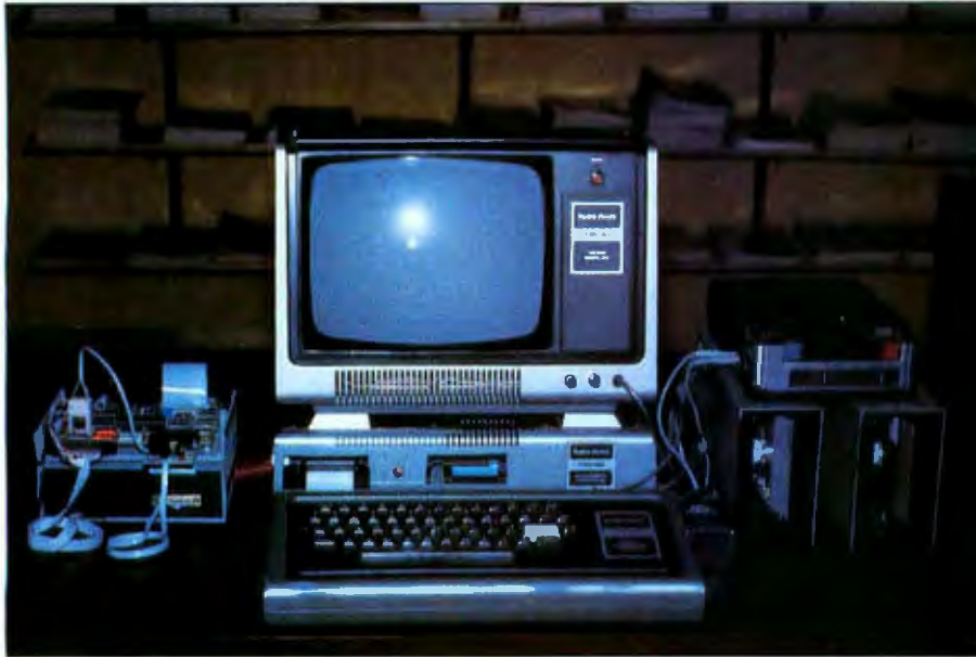
Photo 1: TRS-80 system and test equipment for the COMM-80. The COMM-80 unit under test is on the left with the cover removed and cables attached. The programming techniques employed and described in the testing of this unit are applicable to many other computer-control applications.
