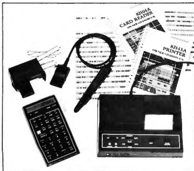
Photo 1: Components of the Hewlett-Packard HP-41C calculator system. Shown here are the calculator itself and three peripheral devices: a magnetic-card reader, a wand for reading printed bar codes, and a thermal dot-matrix printer. The peripheral units plug into four ports at the top of the calculator, which can also receive modules containing additional memory or precoded applications programs. The HP-41C alone costs about $300; a system including all three peripheral devices and two memory or applications modules is about $1000. (Photo by Ed Crabtree.)
