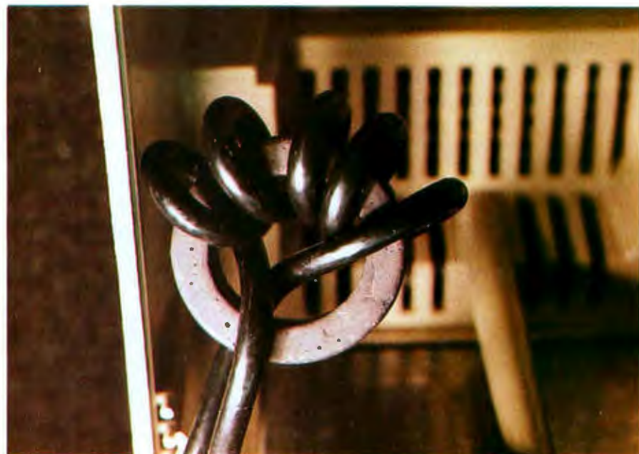
Photo 8: To reduce any high-frequency harmonics that might radiate from the video-monitor cable, a toroidal ferrite core may be wrapped in the line.
