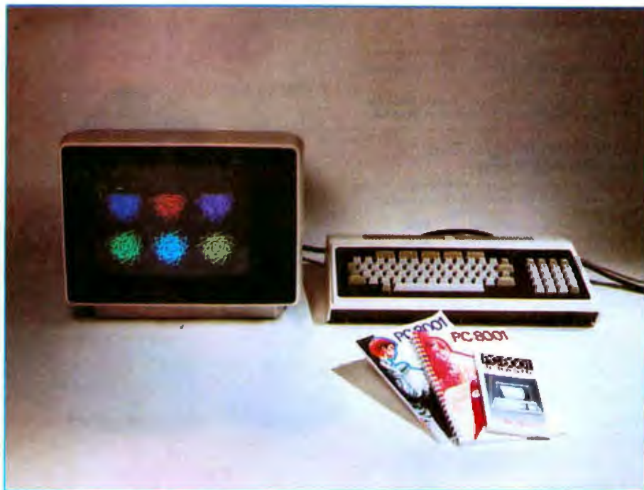
Photo 1: The NEC PC-8001 personal computer system. Shown here is the basic system: high-resolution color monitor, keyboard unit, and documentation (reference manual, BASIC manual, and BASIC reference card).
