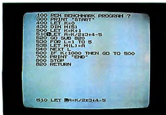
Photo 3: Editing on the ZX80. The cursor (at line 510 at the top of the screen) can be moved via arrow keys to different lines of the program. When the Edit key is pressed, the line being pointed to is copied at the bottom of the screen, where it can be edited. The cursor on the bottom line can be moved right and left; characters can be deleted or inserted at the current cursor position. When the Newline key is pressed, changes made in this line are added to the existing program.
