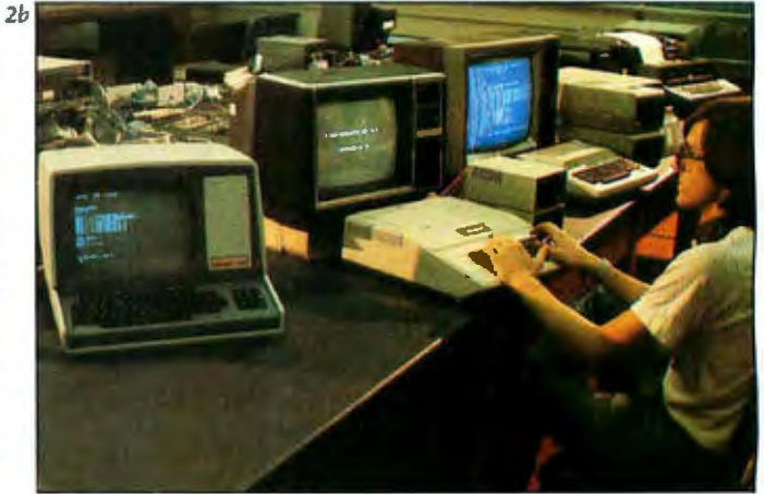
Photo 2: The equipment currently available in the Solo/NET/works laboratory. The terminal at the lower left in Photo 2a is used for the WAG display (as explained in the text). To its right is the IMSAI 5-100 computer that emulates the unrooted-tree network and performs the managerial WAG functions. Further to the right are the system console and bus-status monitor; the other microprocessors operate as nodes in the network. Photo 2b shows MATSRCH designer Ivan Zatkovitch using an Apple II computer in a version of the game that requires only one player.
