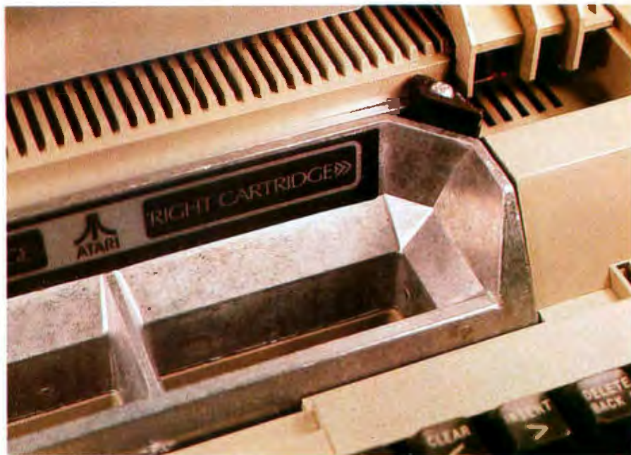
Photo 7: The Atari computers allow the user to plug in special game and business program cartridges. These ROM packs (read-only-memory modules), which are connected directly to the processor bus, must also be kept within the shield when the computer is running. This is accomplished using a special molded, 1/8-inch (9.5 mm)-thick socket that is electrically part of the shield. A plate of aluminum with conductive gasket material around the edges is attached to the cover. When the cover is closed, the memory is completely shielded and virtually no electrical noise is emitted.
