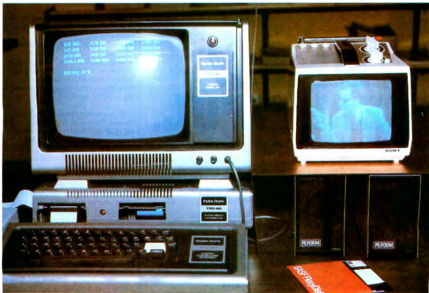
Photo 1b: Demonstration of the effects of shielding. We have added a line filter to eliminate conductive interference to the setup of photo 1a. In addition, two grounded copper sheets, one under the portable TV set and one to the left of it against the side of the TRS-80 video monitor, protect the TV set from radiated noise. The results can be seen as greatly improved picture quality.
