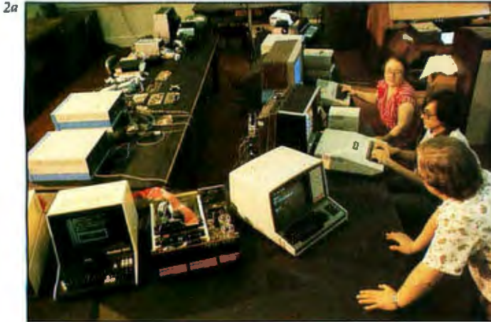
Photo 2: The equipment currently available in the Solo/NET/works laboratory. The terminal at the lower left in Photo 2a is used for the WAG display (as explained in the text). To its right is the IMSAI 5-100 computer that emulates the unrooted-tree network and performs the managerial WAG functions. Further to the right are the system console and bus-status monitor; the other microprocessors operate as nodes in the network. Photo 2b shows MATSRCH designer Ivan Zatkovitch using an Apple II computer in a version of the game that requires only one player.
