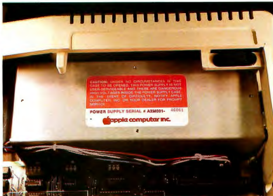
Photo 4: Switching-type power supplies, which use high-frequency pulse-width-modulated waveforms, are a potential source of noise. Most often they are contained in shielded enclosures, as in the Apple II, to eliminate possibly interfering radiation.
