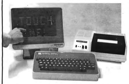
The VuePoint touch-input terminal is 7 cm (2¾ inches) thick and has a 12-line by 40-character flat-panel display. VuePoint's controller provides for up to fifty-one pages of information. A response is sent to the host computer by finger contact to any one of 240 discrete touch-sensitive locations of the display screen. Communication is by selectable 300 to 19,200 bps
