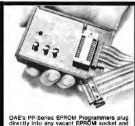
OAE's PP-Series EPROM Programmers plug directly into any vacant EPROM socket and allow you to transfer data directly from RAM to EPROMs. No additional power supplies are required. All timing & control sequences are handled by the programmer. Each unit includes internal DC to DC switching regulator, ZIF and 4 ft. ribbon cable terminated with a 24 pin plug. Programmers are available for all EPROMs from 2708's thru 2532's.
