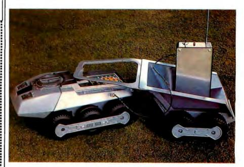
**Photo 11:** When the electronic hardware has been built and is fully operational, the Big Trak Transport (a cargo trailer) provides a convenient method for dragging the wireless communication interface along.
