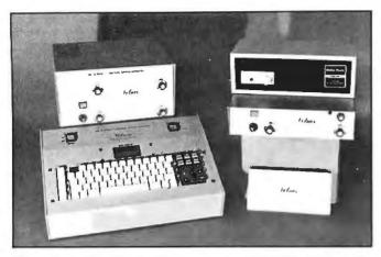
Photo 1: A selection of voice synthesizers. Top left: Votrax ML-I multilingual synthesizer. Bottom left: phonetic keyboard for controlling a synthesizer without the use of a computer. Right top to bottom: Radio Shack TRS-80 Voice Synthesizer, Votrax VS6 synthesizer, Votrax VSK single-board voice synthesizer. Not shown: Votrax SC01 single-chip voice synthesizer.
