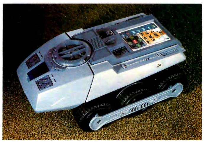
Photo 1: The Big Trak microprocessor-controlled, user-programmable tank, sold by the Milton-Bradley Company.
