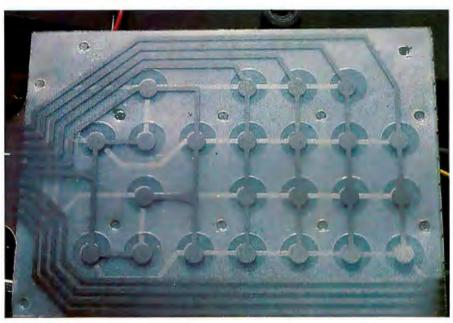
**Photo 4:** A rear view of the keypad, showing its construction. The keypad consists of two plastic sheets containing photo-etched conductors separated by a layer of insulation. At the locations of the function keys, the insulation has a circular cutout through which the two conductive layers can touch when pressure is applied.
