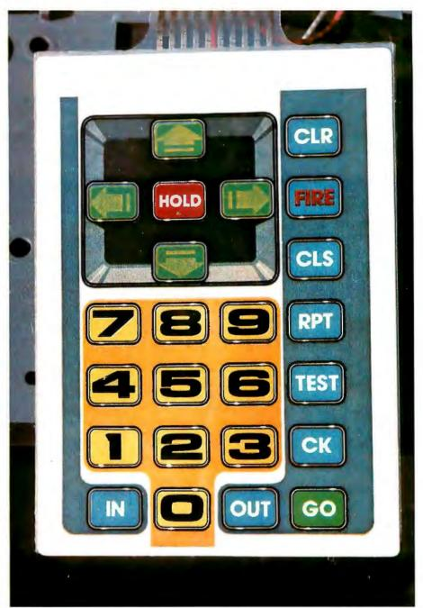
Photo 3: Commands are entered into Big Trak's memory through this keypad on the top of the tank.
