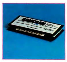
Photo 1: The Axlon RAMCRAM memory cartridge for the Atari 400 or 800.
