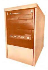
Data Storage Power with 0.5 to 96 Megabytes available. The S100 Bus and SMD disk controller access a variety of hard disk systems:
