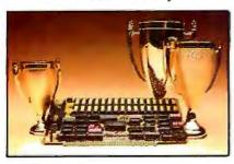
innovative Bank Select switching technique. This enables users to software select up to four totally independent memory banks per board.
