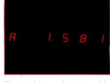
Photo 5: A measured time is read by pressing a letter key on the trainer's hexadecimal keyboard. This is the display's appearance when the A key is pressed to read out the elapsed-time measurement (here 1.581 seconds) stored at memory location A.
