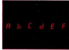
Photo 4: The trainer's six-character LED display after elapsed-time measurements have been logged in all six memory locations, A thru F.
