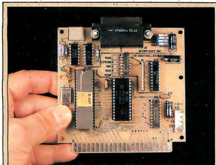
Photo 1: A prototype of the versatile "Circuit Cellar Controller," formally called the Z8-BASIC Microcomputer. The printed-circuit board measures 4 by 4½ inches and has a 44-pin (two-sided 22-pin) edge connector with contacts on 0.156-inch centers. A 2716 or 2732 EPROM can be substituted for the Z6132 Quasi-Static memory, plugging into the same socket.
