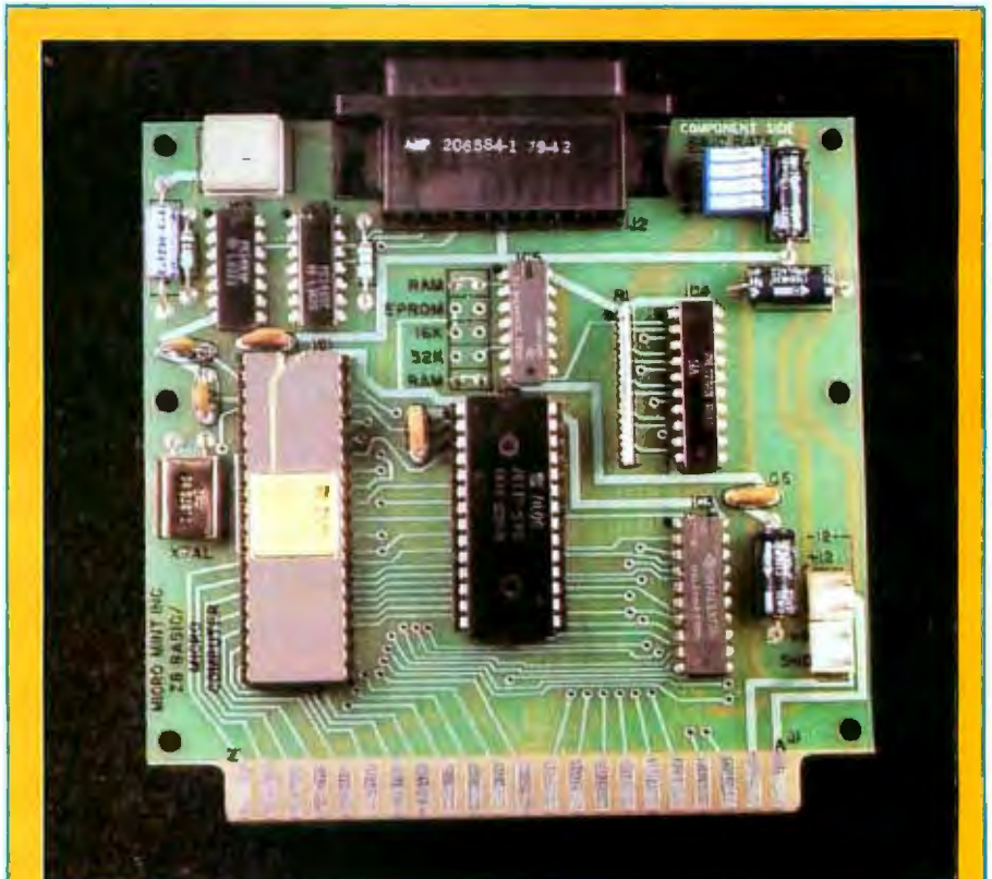
Photo 1: Z8-BASIC Microcomputer. With the two "RAM" jumpers installed, it is configured to operate programs residing in the Z6132 Quasi-Static Memory. A four-position DIP (dual-inline pin) switch (at upper right) sets the serial data rate for communication with a user terminal connected to the DB-25S RS-232C connector on the top center. The reset button is on the top left.
