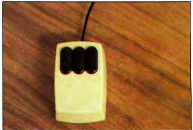
Photo 3: A typical Smalltalk system (photo 3a) and a close-up of the "mouse" (photo 3b), a device that allows you to move an on-screen cursor and select certain options.
