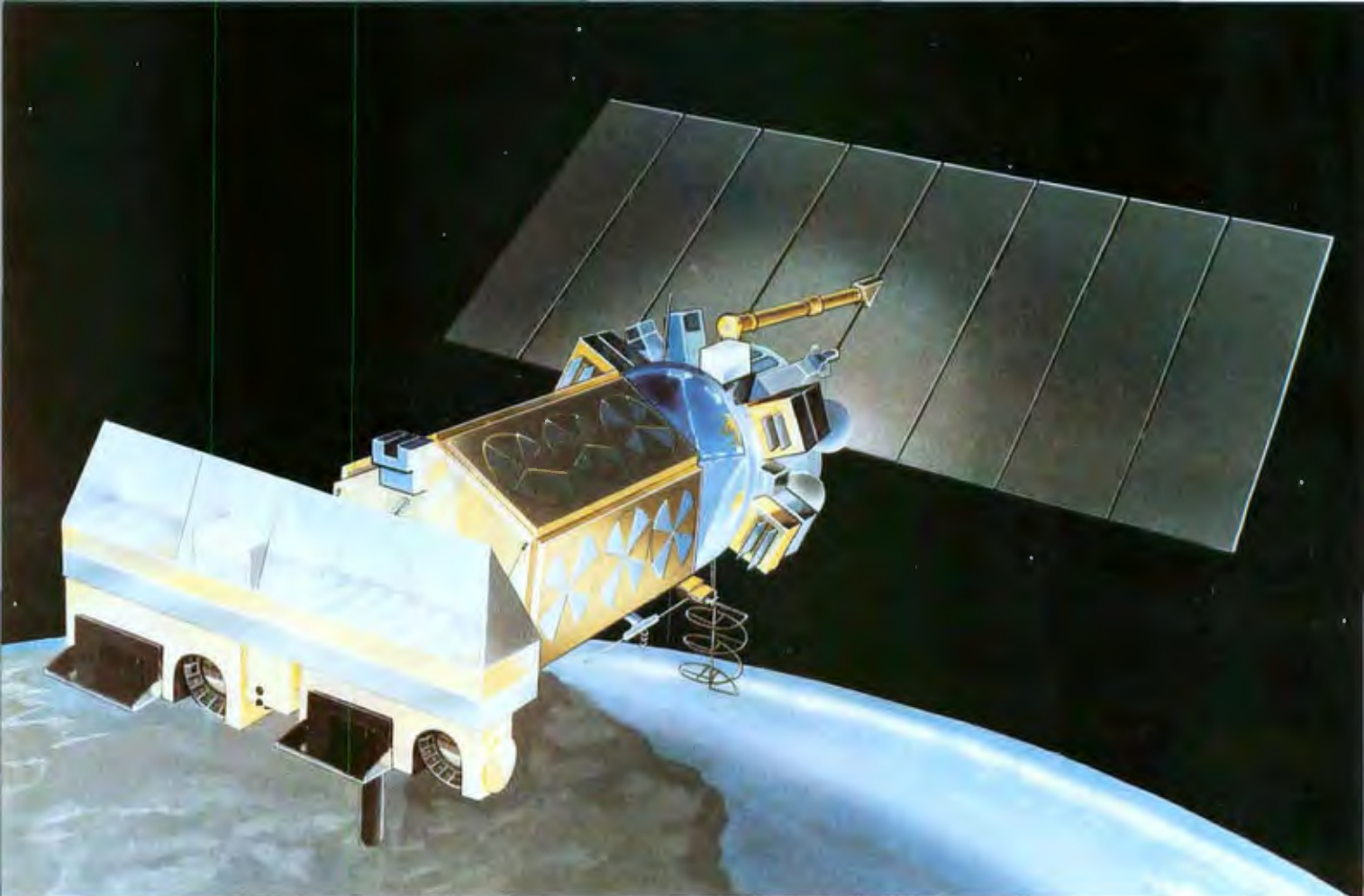
Photo 1: Advanced TIROS-Class Weather Satellite. Used in military and civilian versions, the TIROS satellites have two on-board computers.
