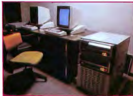
Photo 1: Two of the Xerox Alto personal computers. Each Alto processor is made of medium- and small-scale TTL integrated circuits, and is mounted in a rack beneath two 3-megabyte hard-disk drives. Note that the video displays are taller than they are wide and are similar to a page of paper, rather than a standard television screen.
