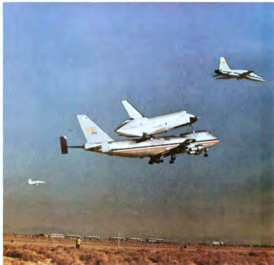
Photo 2: Shuttle Orbiter mounted on transport aircraft. The Orbiter has five on-board computer systems, configured to provide as many as three levels of backup in critical situations. Two chase planes are visible.
