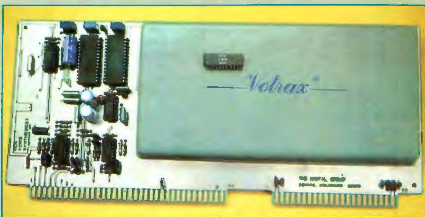
Photo 3: Before the development of the SC-01, Votrax used many medium-scale-integrated circuits and discrete components to perform the same functions. All these components were mounted in modules such as the VSL-type shown. When this particular synthesizer card was purchased three years ago, the price was $600. Compare this both in size and price to the $70 SC-01 (sitting on top).
