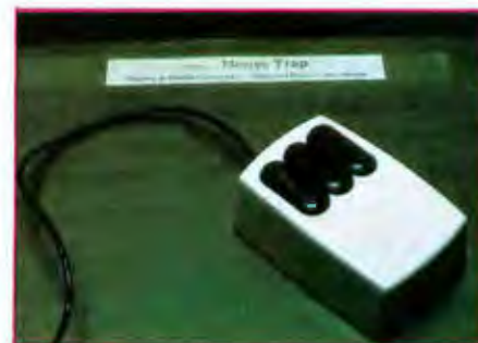
Photo 4: The mouse input device. The operator uses the mouse to control cursor placement on the screen; it detects its own change in position (a joystick relies on absolute position) as the operator rolls it around on a piece of soft plastic. The mouse also has three buttons, called red, yellow, and blue.
