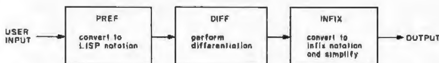
Figure 1: Skeletal structure of the symbolic-differentiating system. Each block represents a recursive function that performs the task denoted within.
