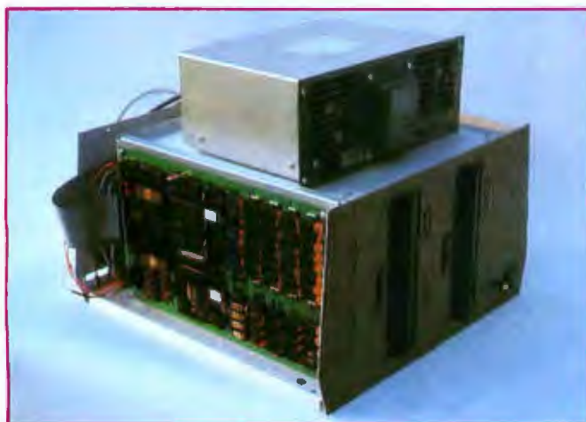
Photo 4: The Big Board in place in the author's system. Resting on top of the cabinet is the power supply, originally built for a Digital Equipment Corporation controller.
