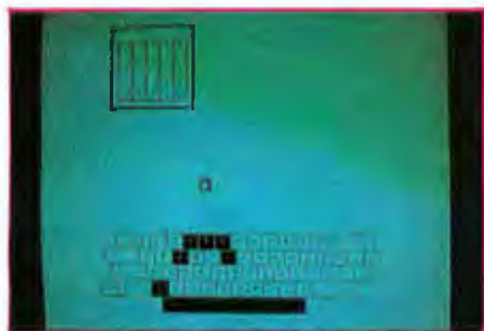
Photo 2: Display from the keyboard-test program. The Alto keyboard has a separate signal line for each key and can thus tell when any number of keys are being pressed simultaneously. In the display, the black keys are being held down. The small square above the keyboard represents the mouse (see photo 4); one mouse key is also pressed.
