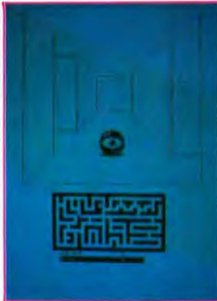
Photo 8: The multiplayer Mazewar game. The eye represents the persona of an opponent. Any Alto on the net can join or leave the game at any time.
