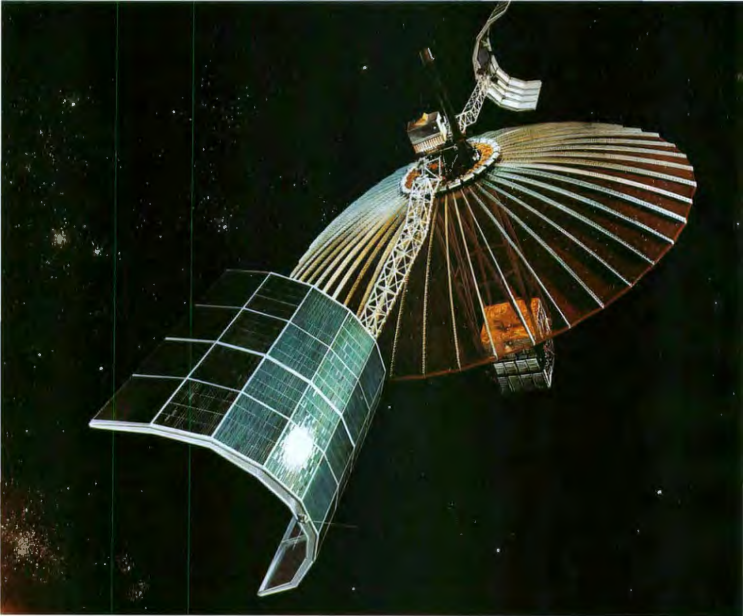
Photo 3: ATS-6 Communications Satellite. Traveling in synchronous orbit, the ATS-6 uses two on-board computers for attitude control.
