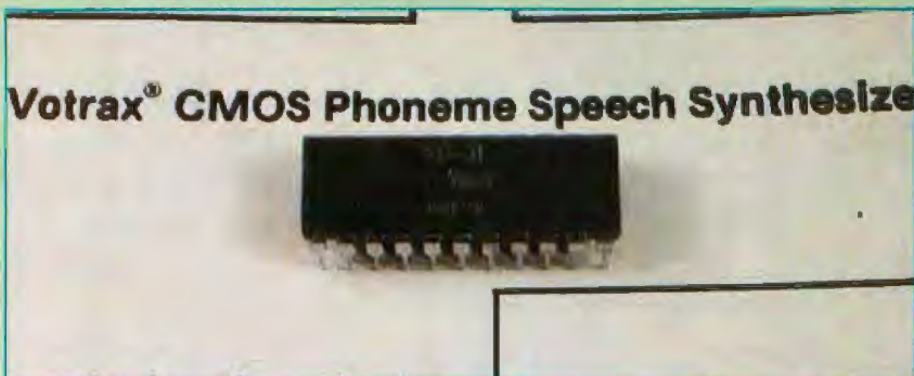
Photo 2: The Votrax SC-01 is a 22-pin CMOS integrated circuit which functions as an electronic model of the human voice.
