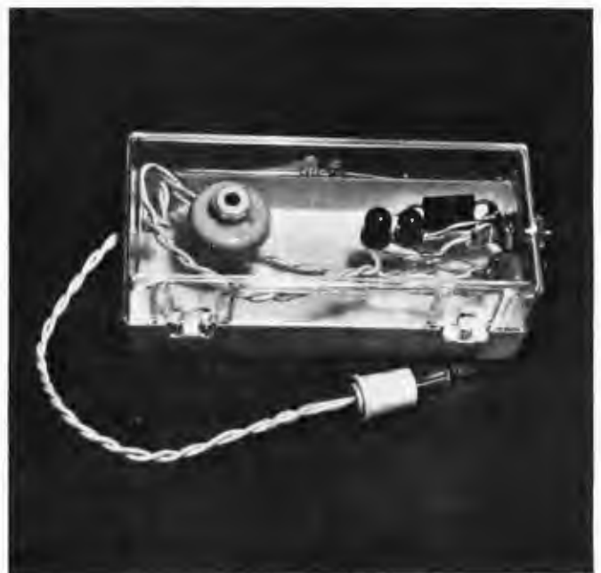
Photo 1: The cassette level indicator built inside a small plastic box.
