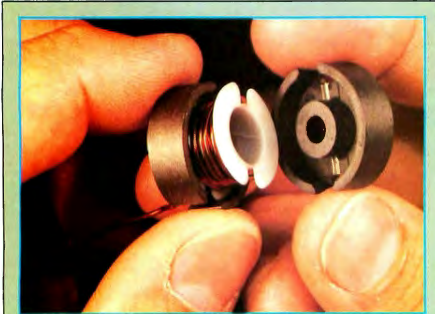
Photo 3: Winding the inductor for the switching supply of figure 6a. The turns of wire are neatly wound around a plastic bobbin, evenly distributed.
