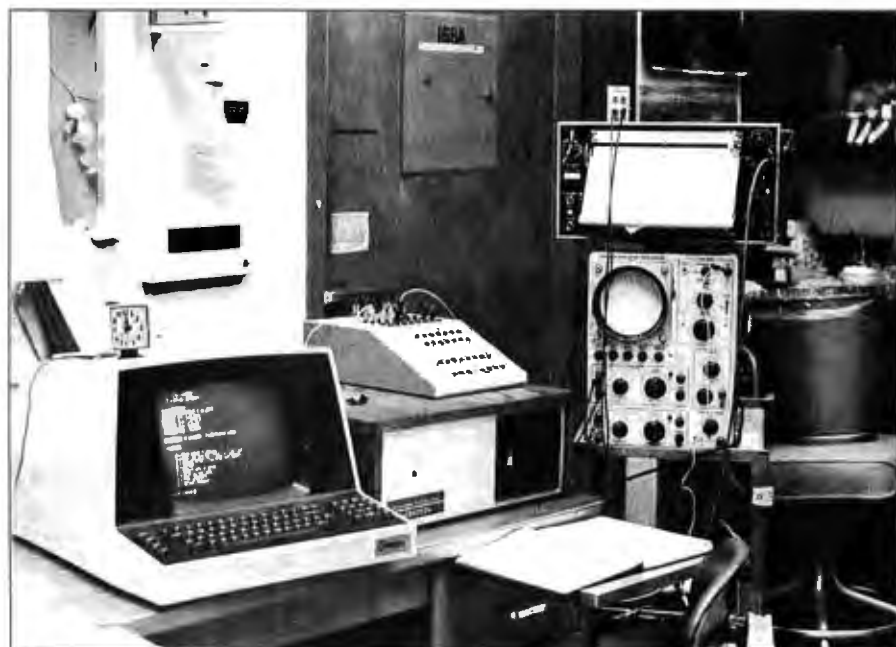
Photo 1: View of the laboratory microcomputer, showing the Soroc video console, Horizon II computer, interface box, and oscilloscope and strip-chart recorder used for graphic display of data. Plant growth transducers and other instruments located in a controlled-temperature room behind the computer are plugged into the interface box on top of the Horizon.
