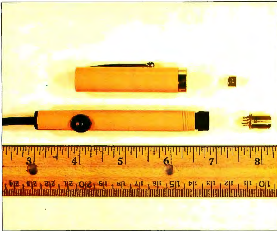
Photo 1: Author's bar-code scanning wand. The wand is based on Hewlett-Packard's HEDS-1000 optical reflective sensor (the metal can with eight pins), and a Schaefer No Nonsense ball-point pen. The calibration cylinder appears at the right of the HEDS-1000 module.
