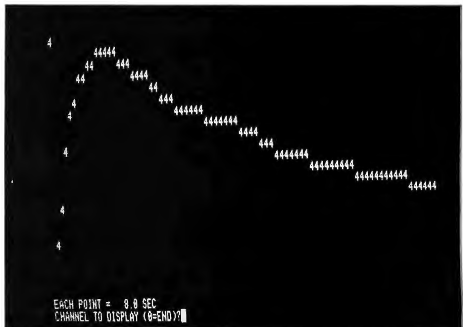
Photo 2: Sample display of data on the Soroc system console using the terminal's direct X-Y cursor-positioning ability.
