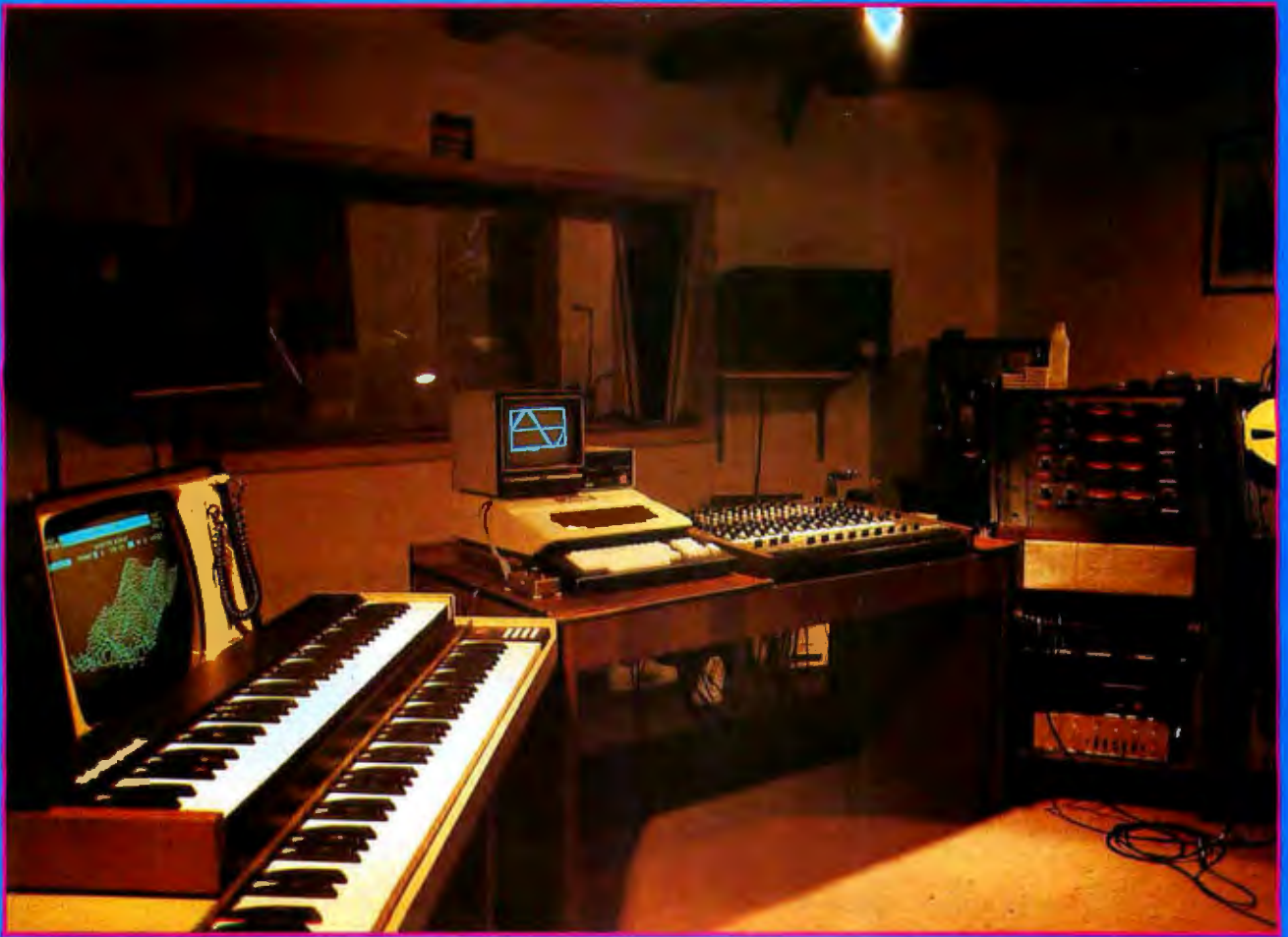
Photo 5: Bill Mauchly's eight-track Linden Studio in Ambler, Pennsylvania. In the foreground is the Fairlight Computer Music Instrument, the alphaSyntauri keyboard on top of the CMI, the monitor, an Apple II with Mountain Computer music synthesizer boards, the Fairlight ASCII keyboard, The Sound Workshop 12-channel mixing console, an Otari eight-track recorder, and various outboard equipment in the rack at lower right. The studio is a 100-year-old barn, and the research lab is located a short distance away. (Photo by Irene Mohler)
