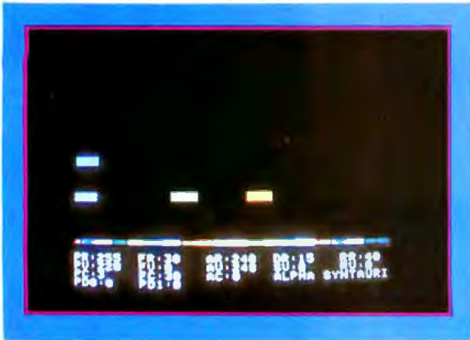
Photo 1: The Envelope Control Screen is shown with a color display of a C major chord. P00 and P01 are live paddle displays of the vibrato and FX controls.
