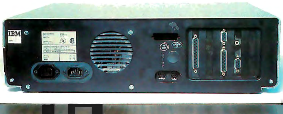
Photo 10: The back panel of the IBM Personal Computer. See the text for a description of the plugs and sockets.
