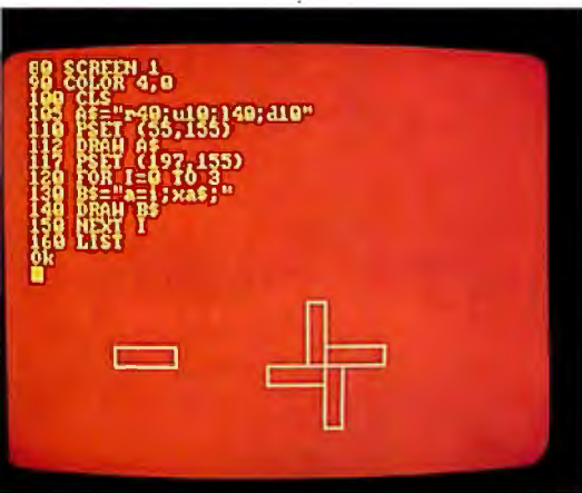
Photo 11: A demonstration of the DRAW command. See the text for details.
