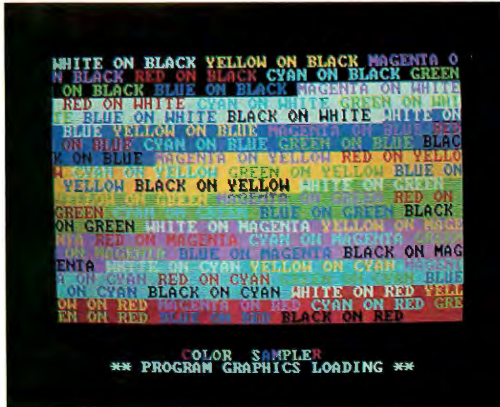
Photo 8: An example showing the independence of foreground and background colors when using the text mode of the color/graphics adapter board.
