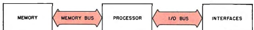
Figure 2: A computer system with an I/O bus in addition to a memory bus. Building in a separate I/O bus frees all the memory-address space for the processor's own use.
