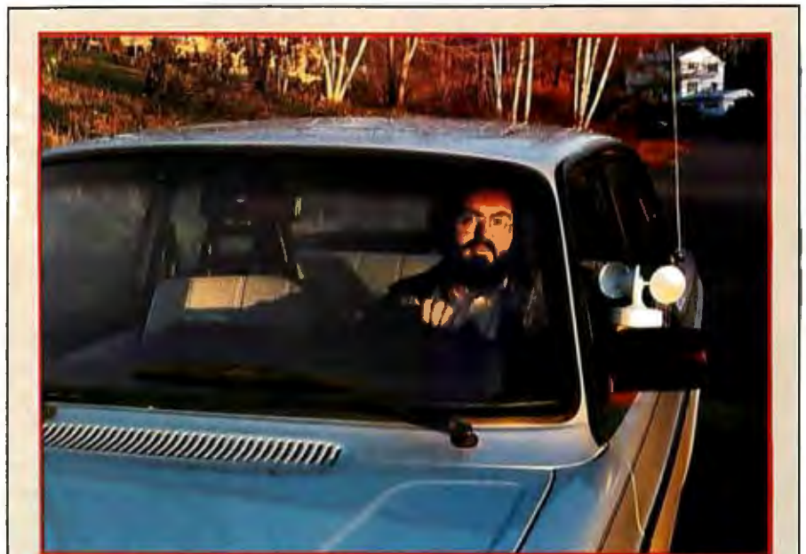
Photo 6: The anemometer was calibrated by moving it relative to still air; holding it out the window of a moving automobile worked quite well. Driving at a known speed, I used the circuit of figure 5 to record its pulses; the characteristic curve is shown in figure 6.
