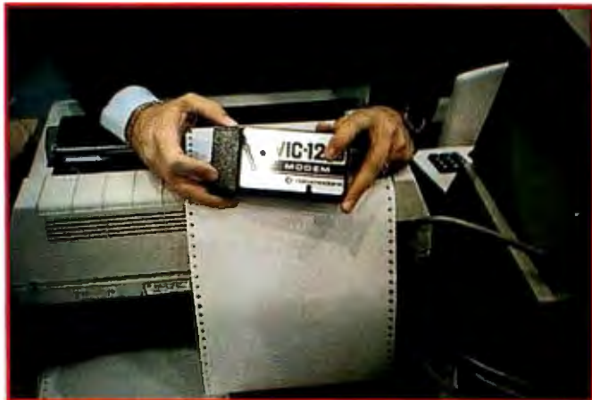
Photo 3: Commodore's new, under-$100 modem for the VIC-20 color computer. The VIC-12 plugs directly into the VIC-20 and features a modular jack.
