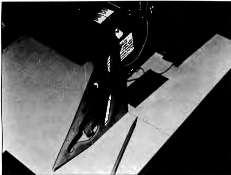
Photo 1: Use a square or a drafting triangle to mark the table directly beneath the center of the knob. Measure the height of the shaft above the table and mark the triangle.
