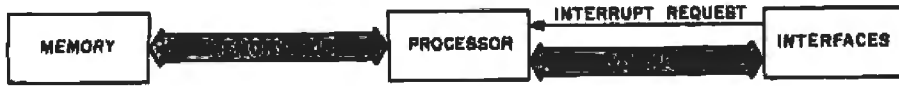
Figure 4: A computer system with memory bus, I/O bus, and added interrupt line. Interrupts allow the processor to start I/O processes, then go on to other tasks. The peripheral uses the interrupt line to indicate readiness for another transaction.
